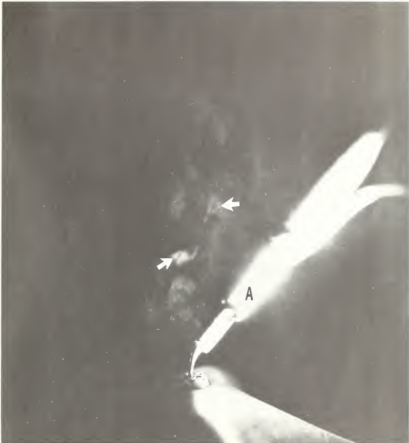
Fig. 1. A cloud of material, arrows, is being emitted from the amalgam at the tip of an ultrasonic amalgam condensing instrument. The particles, also shown in Fig. 3, settle on the instrument handle, A, and may be responsible for some of the haze surrounding the handle.
