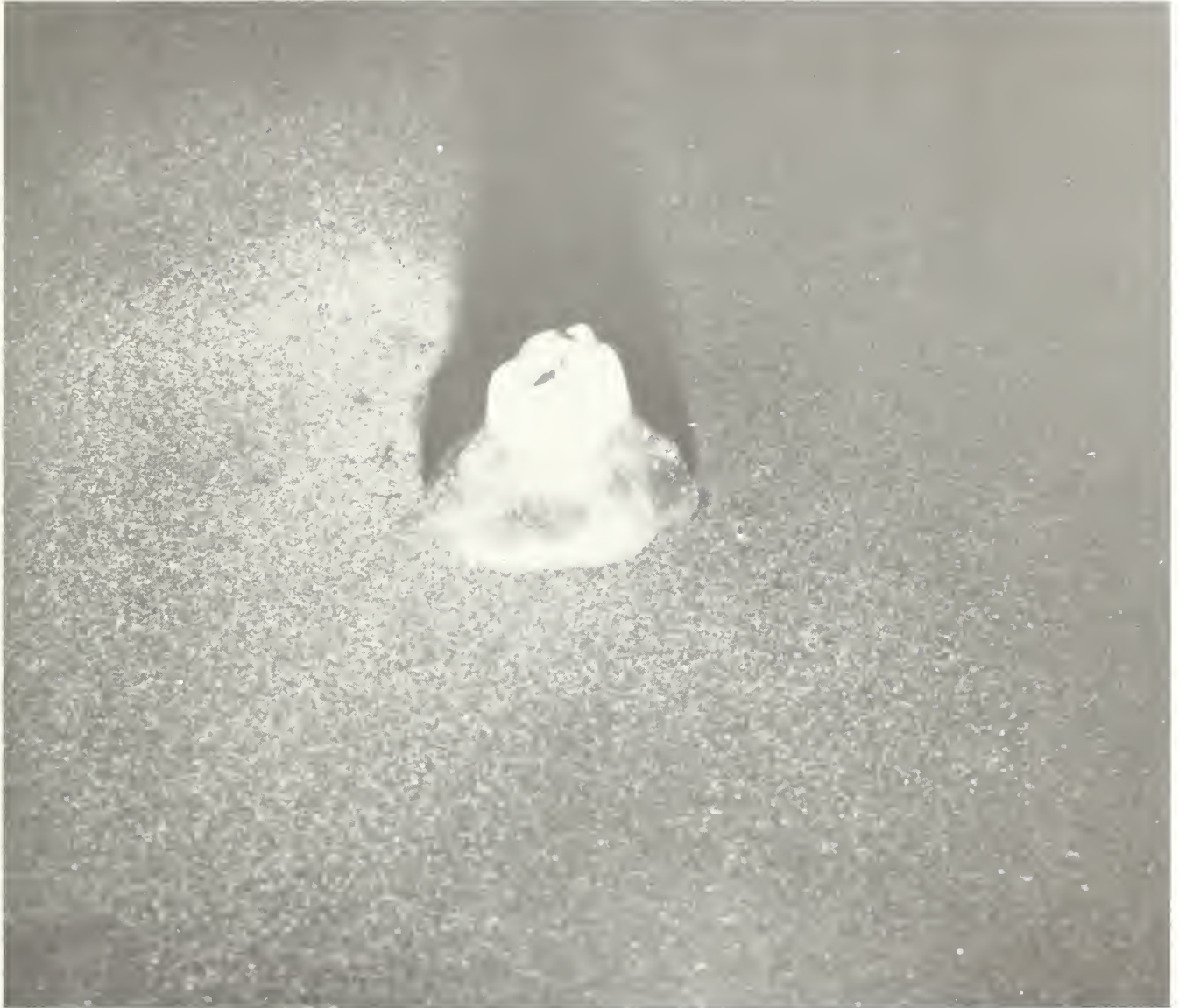
Fig. 3. A porcelain tooth and the surrounding operating field after condensation of 3 amalgam mixes into the tooth. The background is plain black paper. Note the great number of mercury and alloy particles that have been deposited around the operating site. The dark area behind the tooth is a shadow caused by the oblique lighting used in making the photograph.
