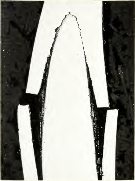
(10b) 250X View of top of bend in wire appearing in Figure 10a. Separation of nickel layer from basket wire is evident.
