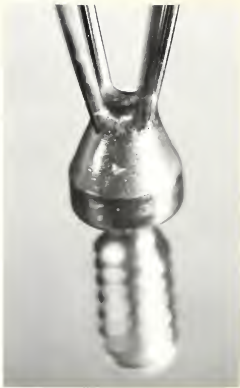
(a) 12X Filiform tip end of unused stone dislodger shown in Figure 1a.
