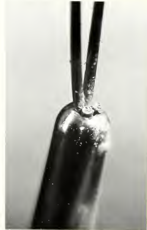
(d) 12X Flexible cable end of used stone dislodger shown in Figure 1c.
