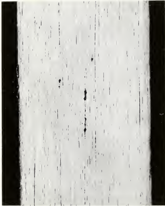
Figure 5. Fibrous appearance of basket wire in spring temper condition. Sample taken from unused stone dislodger appearing in Figure 1a. Etched in 20% HCl, 5% HNO 3 .
