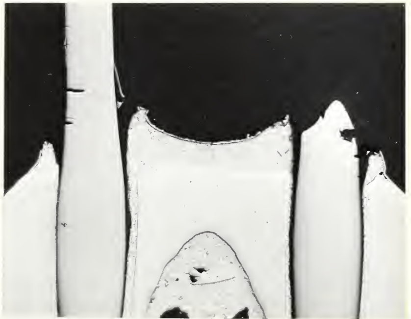
(8b) 50X Solder bead appearing in Figure 8a at point where basket wires enter filiform tip.
