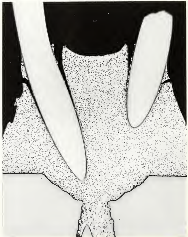
Figure 6. Cross-sectional view of soldered joint within filiform tip. Sample taken from unused stone dislodger appearing in Figure 1a.
