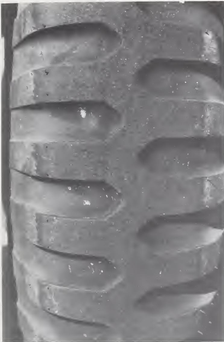
Figure A-1. Characteristic tread element pattern of tire A (standard Army tire). The nominal new tread depth for this tire was 21/32 inch. Shore hardness values ranging from 51-60 were observed with the average being 57.
