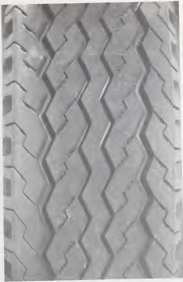
Figure A-2. Characteristic tread element pattern of tire B (commercial rib tire). The nominal new tread depth for this tire was 16/32 inch. Shore hardness values ranging from 60-64 were observed with the average being 61.
