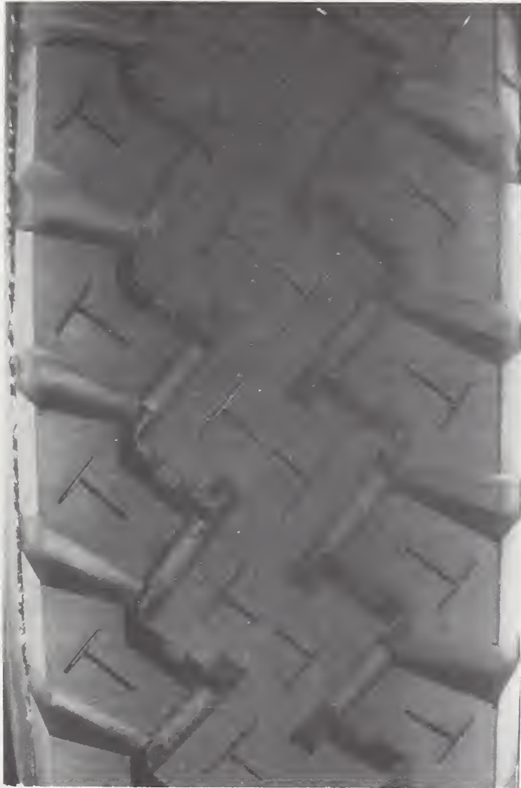
Figure A-4. Characteristic tread element pattern of tire D (commercial cross-bar tire). The nominal new tread depth for this tire was 19/32 inch. Shore hardness values ranging from 61-66 were observed with the average being 64.
