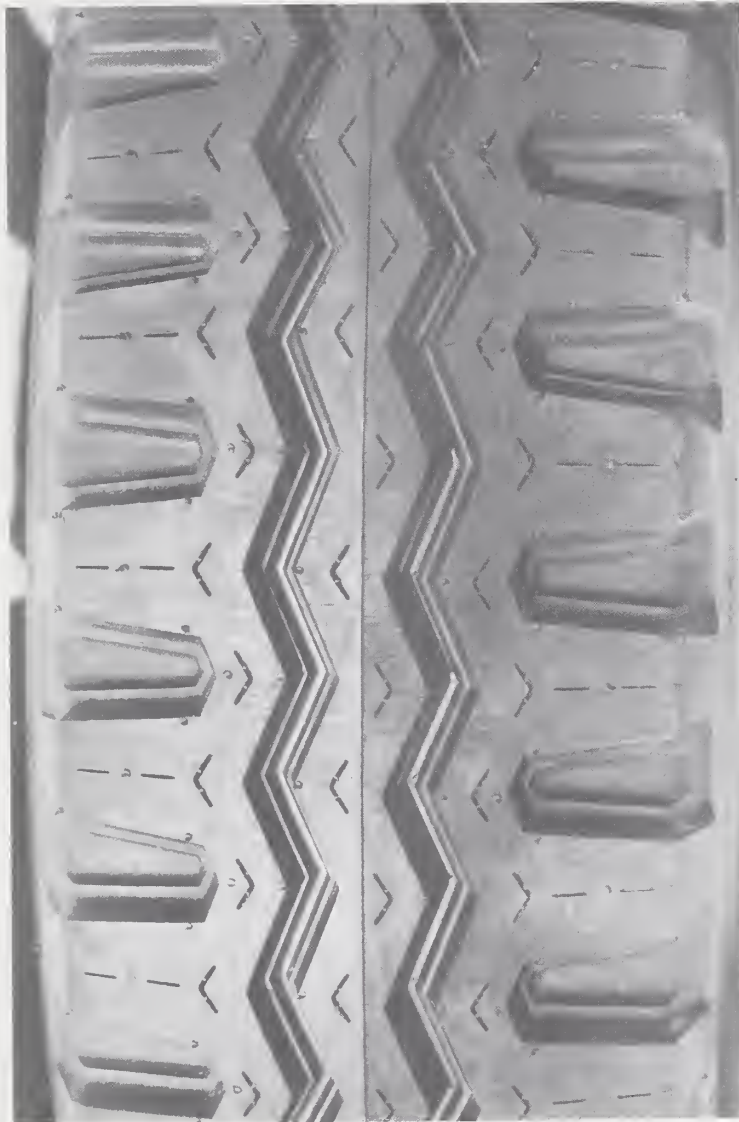
Figure A-3. Characteristic tread element pattern of tire C (Army-retread tire). The nominal new tread depth for this tire was 20/32 inch. Shore hardness values ranging from 58-64 were observed with the average being 62.
