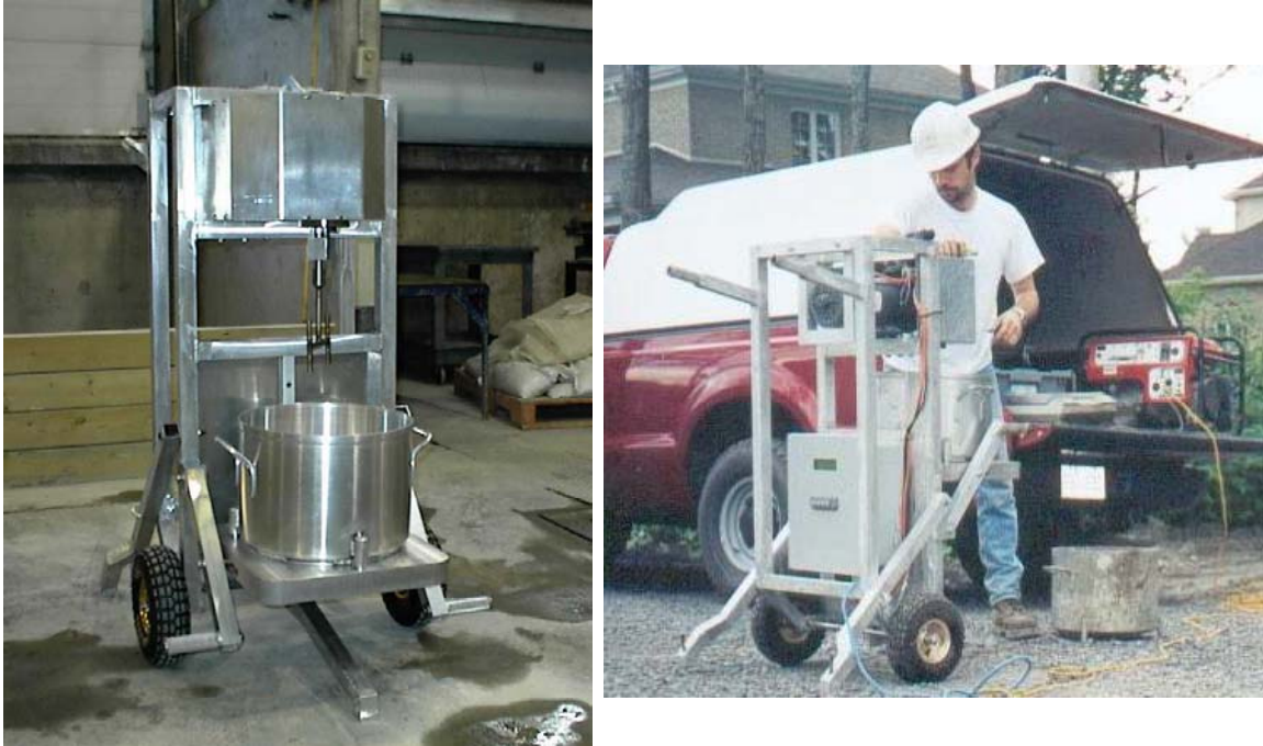
Figure 10: Picture of portable IBB Rheometer (a) in the lab and (b) on a construction site
