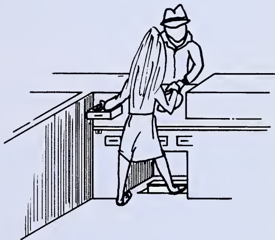
A holdup device is a manually actuated switch set off by an employee during a holdup.
