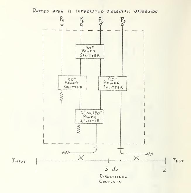
Figure 2. Schematic of six-port network.
