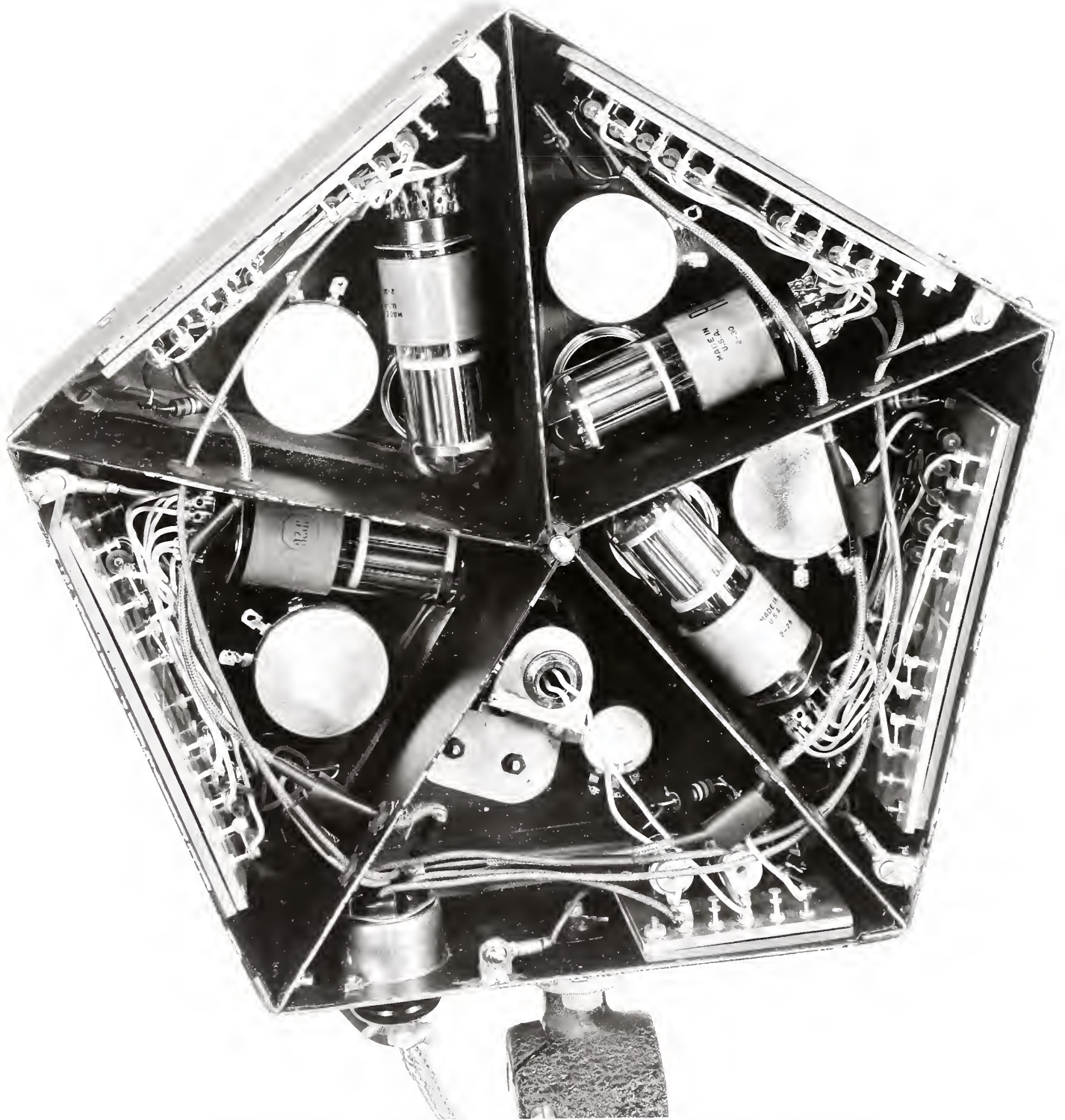
FIG. 6 SPECTRORADIOMETER RECEIVER, REAR VIEW OF INTERIOR
