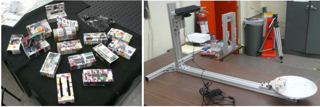
Figure 10. Shows the artifacts used in the challenge and the ground truth rig with the sensor mounted at top left. [Permission granted by the author [41] to use the Figure]
