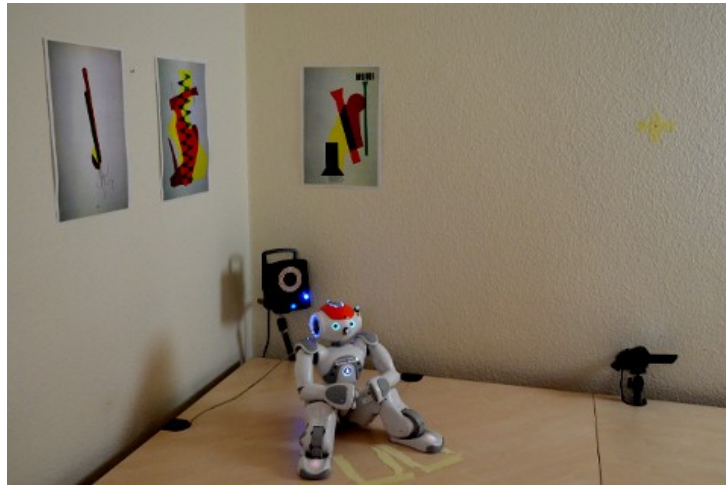
Figure 18. Figure shows the Nao robot and the Vicon MoCap framework for acquisition of multimodal human-robot interaction datasets. [Permission granted by the author [34] to use the Figure]
