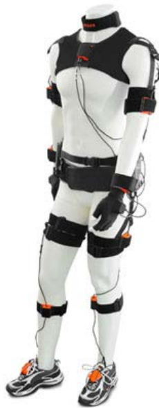
Figure 19. Shows an inertial motion capture system for tracking and motion capture. [Permission granted by the company [73] to use the Figure]
