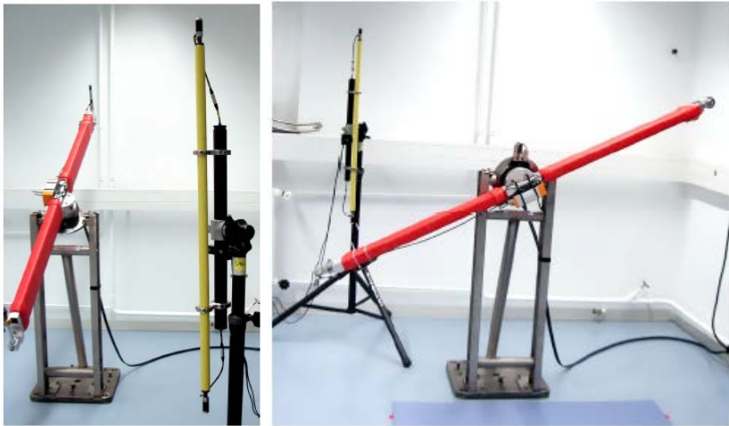
Figure 12. The rotating arm and the scale bar, for dynamic repeatability comparisons of tracking systems, by using four iGPS transmitters arranged around the rotating arm and a scale bar used for bundling. [Permission granted by the author [50] to use the Figure]
