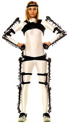
Figure 20. Shows a mechanical motion capture system. [Permission granted by the company [82] to use the Figure]
