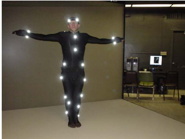
Figure 17. Reflective markers are attached to the surface of a human or object to identify and capture the 3D motion. (Image from http://www.flickr.com/photos/funksoup/88138710/ Creative commons))
