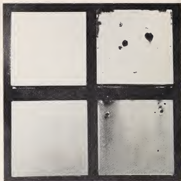
FIGURE 3. Four panels after 15 years of exposure at Atlantic City.
