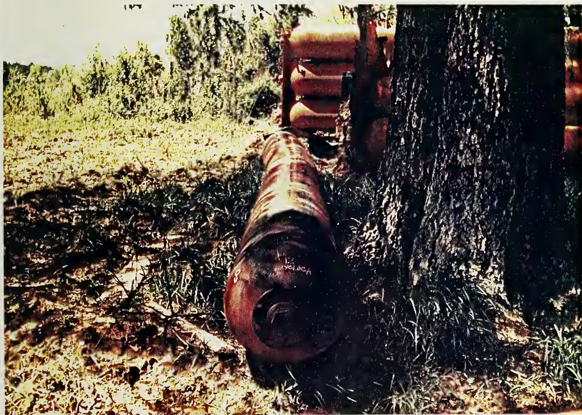
Figure 10b. Bowing of cylinder Number 8 due to the blow resulting in the hit mark shown in Figure 10a.
