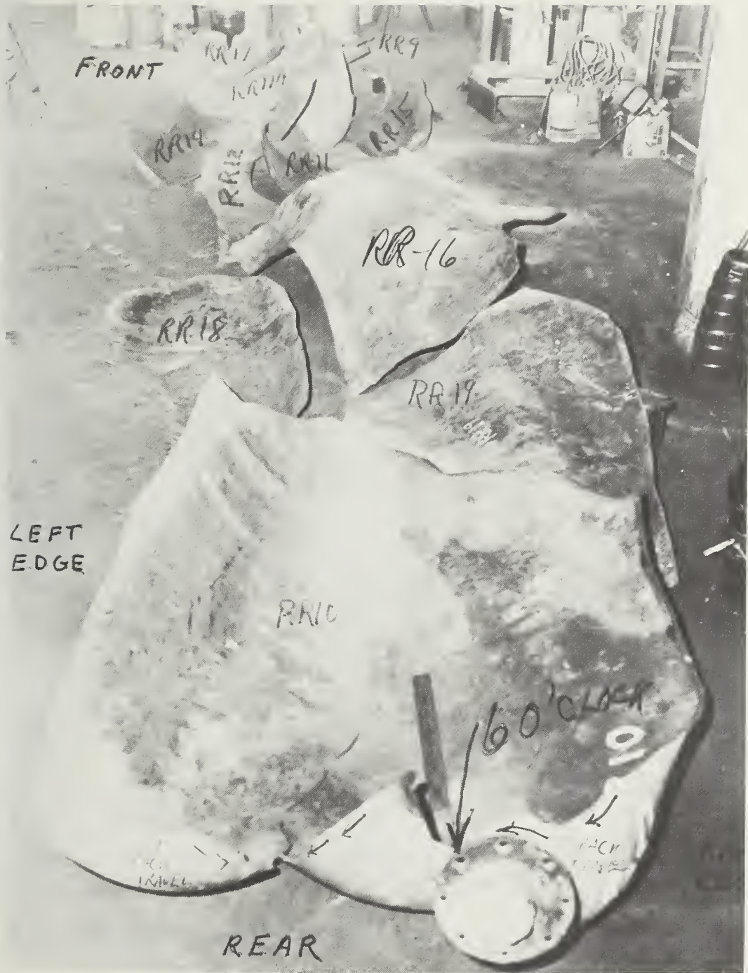
Figure 2a. Eleven pieces of cylinder 9959 laid out on the floor at Gladstone Laboratories, Inc. The rear head is in the foreground. (Photo courtesy of M. Bolinger, Jr., Gladstone Laboratories, Inc., Cincinnati, Ohio).
