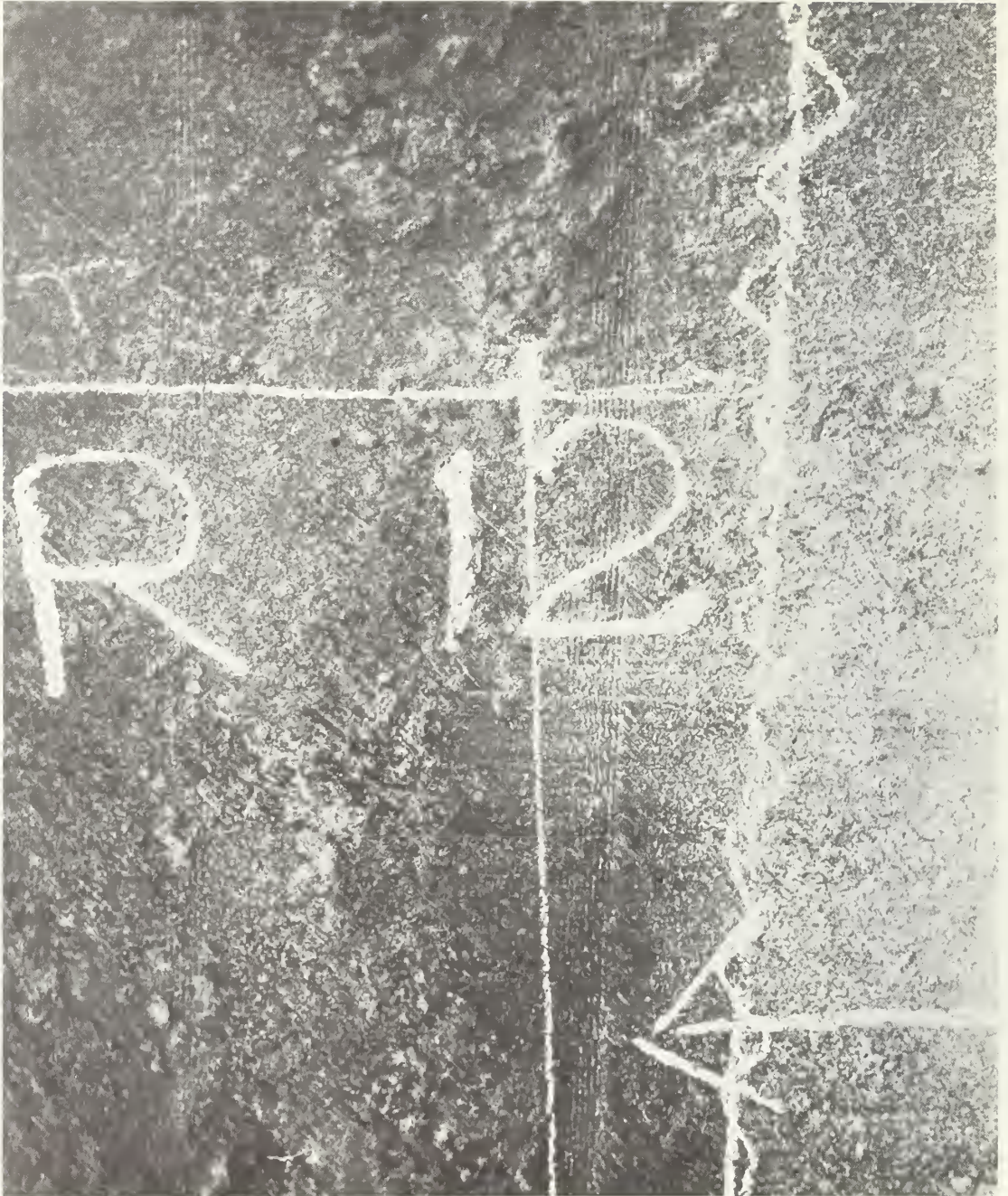
Figure 18b. A view of piece RR-12 showing sets of parallel lines running in the circumferential direction. (Photo courtesy of M. Bolinger, Jr., Gladstone Laboratories, Inc., Cincinnati, Ohio.)
