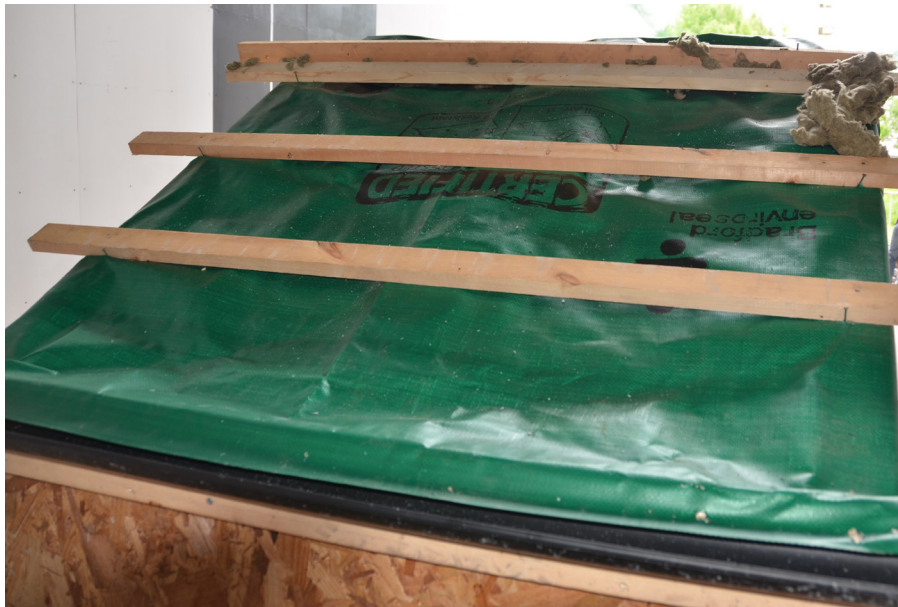
Figure 3. Custom Assembly used to Mount the Various Tile Roofing Assemblies. The Sarking (green material) as well as the Battens used to Support the Tiles are Clearly Visible. In this Picture the Batten Spacing was Adjusted for Terracotta Tiles (flat tiles).
