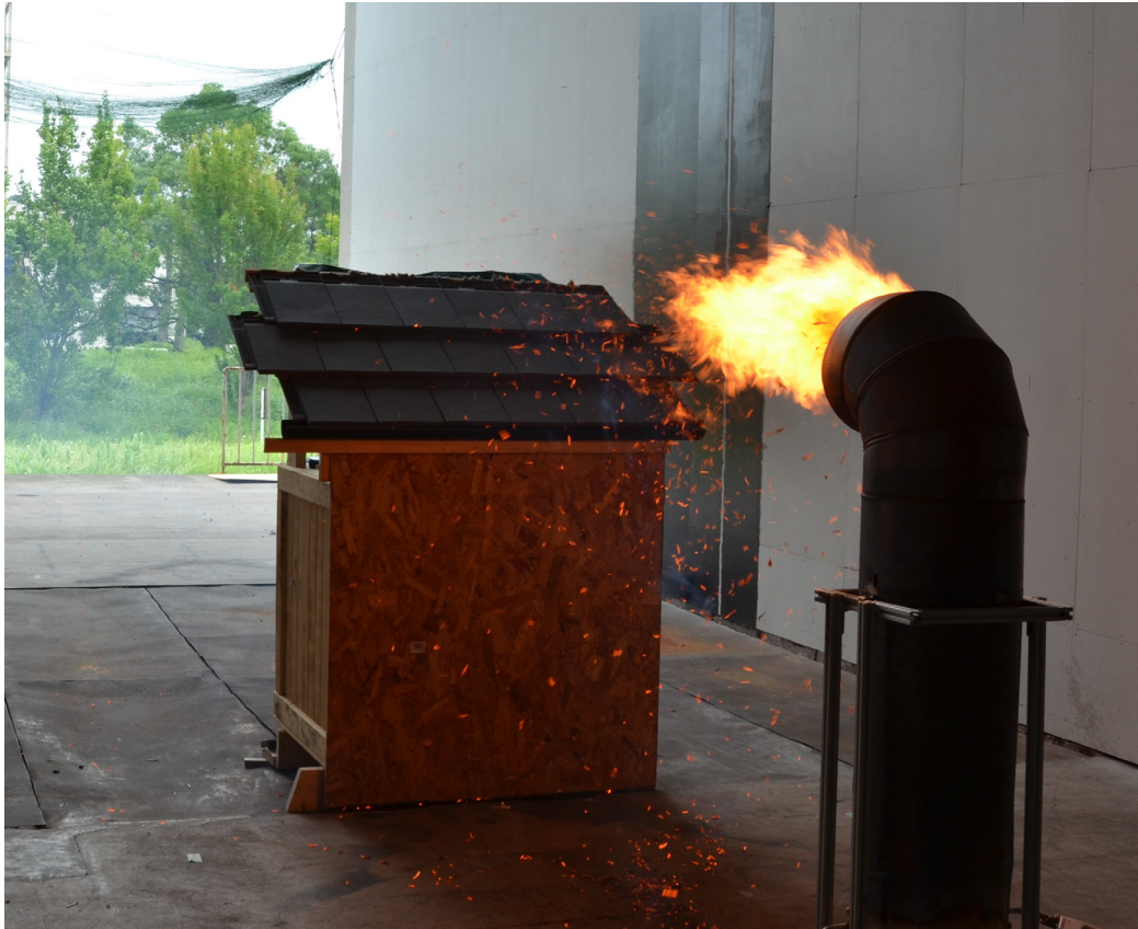
Figure 8. Typical Experiments Exposing Terracotta Tile Roofing Assembly (flat tiles in this image). The Wind Tunnel Speed was 9 m/s and the Roofing Assembly was Located 2.0 m from the NIST Dragon. The Average Total Firebrand Mass Flux was 10 \text{ g/m}^2\text{s} .
