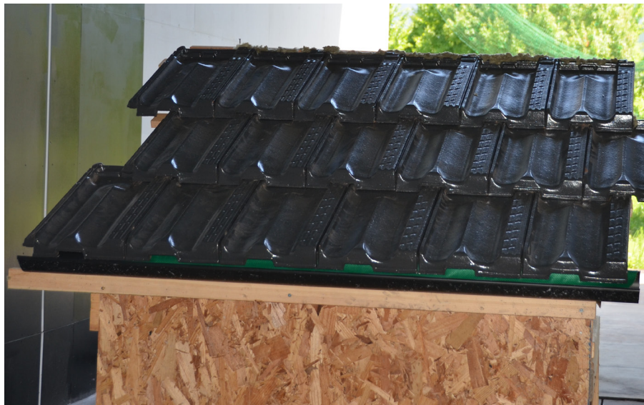
Figure 6. Terracotta Tiles Roofing Assembly (flat tile) Exposed to Wind-Driven Firebrand Showers. The Dimensions of Each Tile were 425 mm long by 265 mm wide. The Height, from the Wind Tunnel Floor to the Base of the Gutter of Roof Deck was 1250 mm.
