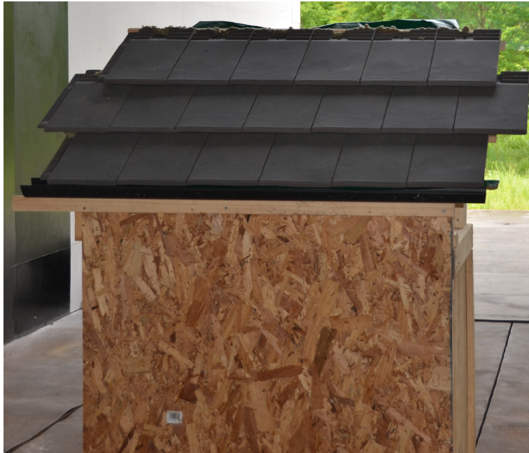
Figure 6. Terracotta Tiles Roofing Assembly (flat tile) Exposed to Wind-Driven Firebrand Showers. The Dimensions of Each Tile were 425 mm long by 265 mm wide. The Height, from the Wind Tunnel Floor to the Base of the Gutter of Roof Deck was 1250 mm.
