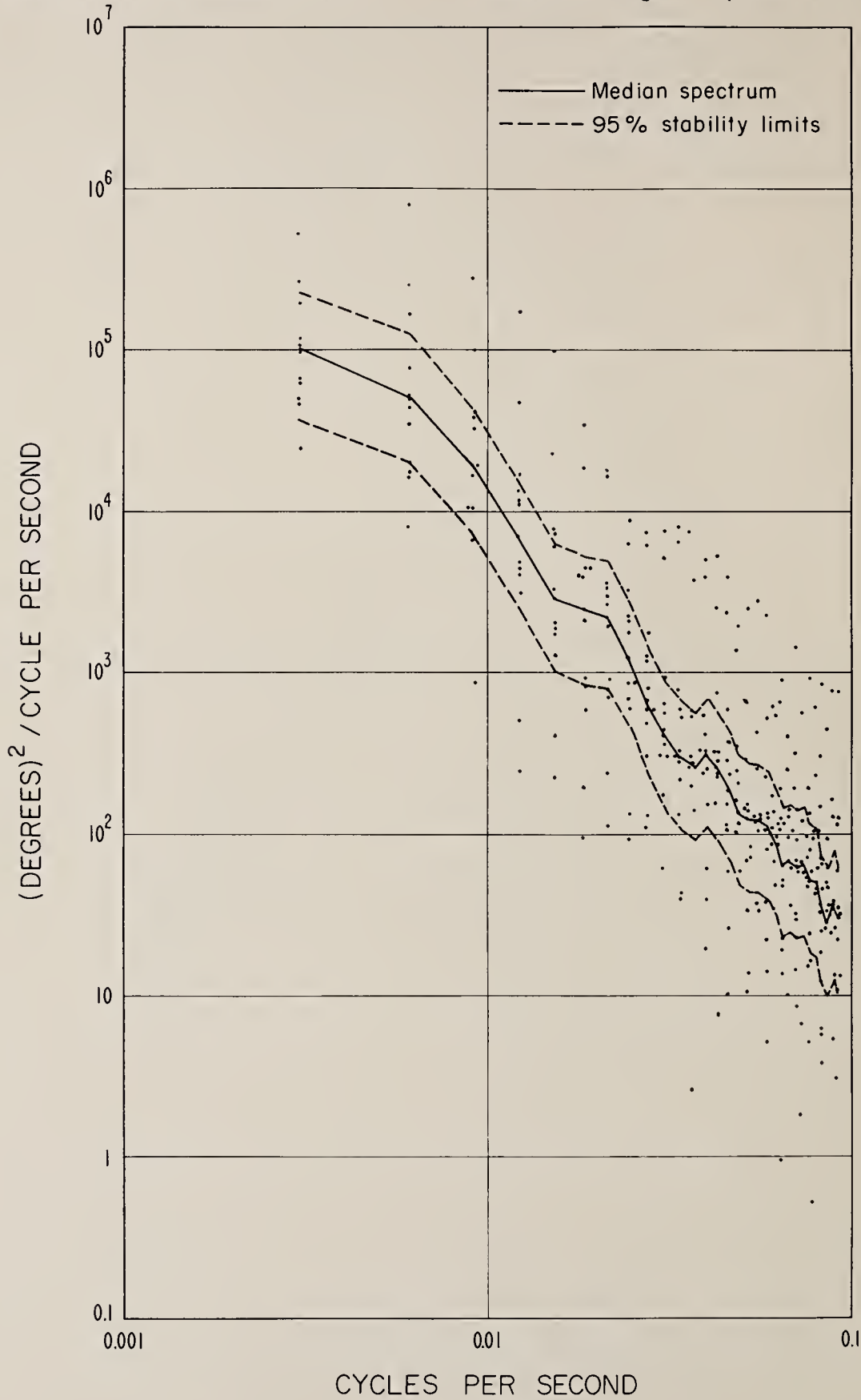
FIGURE 40. Power spectra of 9,414 Mc/s phase difference variations. (Data samples 48 to 60, incl., from ABH recording period)
