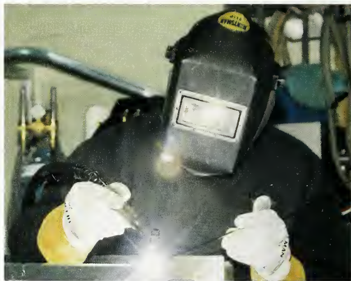
FIGURE 6. NCNR Mechanical Engineering Technician Scott Slifer welds the aluminum moderator vessel for the advanced hydrogen cold source.
