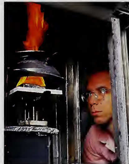
Cone calorimeter being used to measure effect of fire retardants
