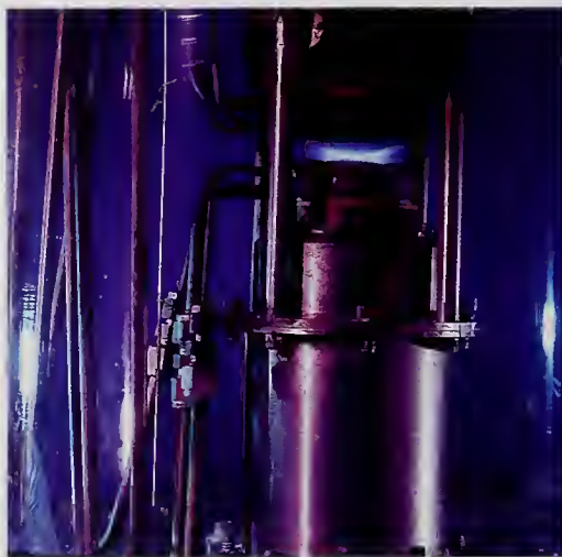
Stabilized flame for measuring refrigerant flammability
