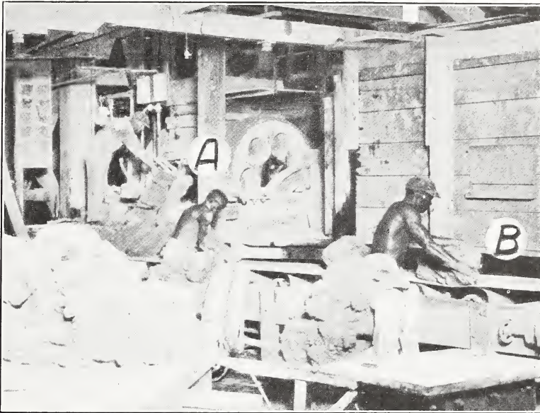
FIG. 13.—Wet pan in which the mixtures of clay, grog, and other materials which may be used in the manufacture of brick are ground and tempered with water to a plastic mass
