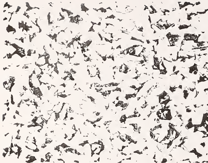
Figure 37. Ferrite–pearlite microstructure of the 14-mm-thick VT medium-carbon steel cooled to ambient temperature after rolling (200 \times ).
