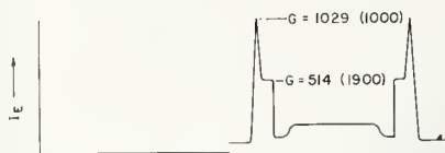
b. Current gain for 10-keV electrons with the signal taken from the emitter with the base and collector grounded.
