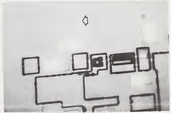
Figure 74. Portion of a quad 2-input NAND gate including a functional gate on the left and a nonfunctional gate on the right.
