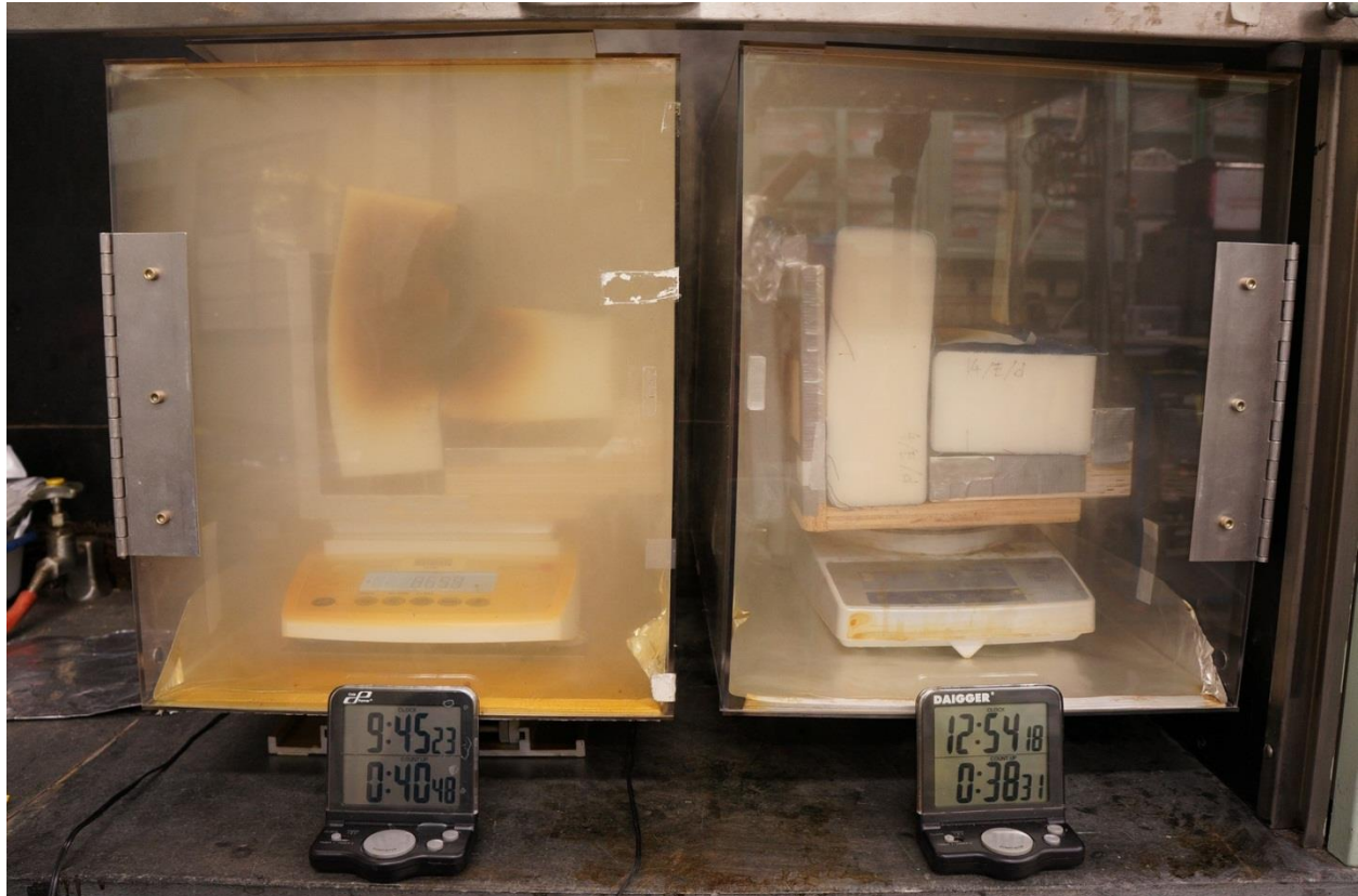
Figure 9. Photograph of the closed (right) and open (left) mockups after about (39 to 40) min from the beginning of the test. Foam F is used for both mockups.
