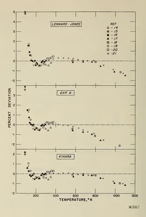
Fig. 2. Percentage deviation plots  $\left[ \left( \frac{\eta_{\text{exp}} - \eta_{\text{calc}}}{\eta_{\text{calc}}} \right) \times 100 \right]$  of experimental and calculated viscosity coefficients for the three potential functions using the best values from Table II (Note: data from Ref. 14 is obtained by extrapolation to a pressure of one atmosphere).
