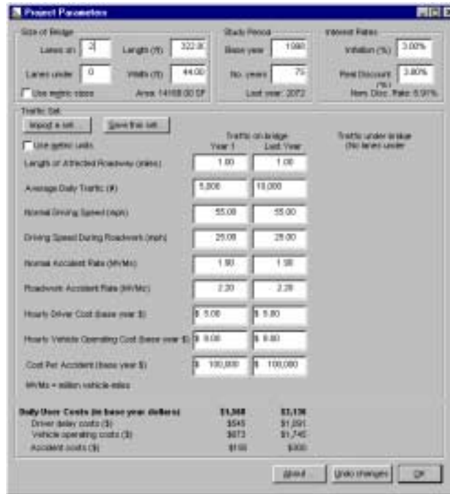
Figure 36. Project Parameters Window
