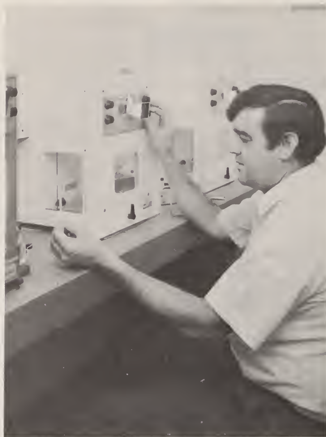
Figure 5. Gravimetric calibration of permeation tubes.
