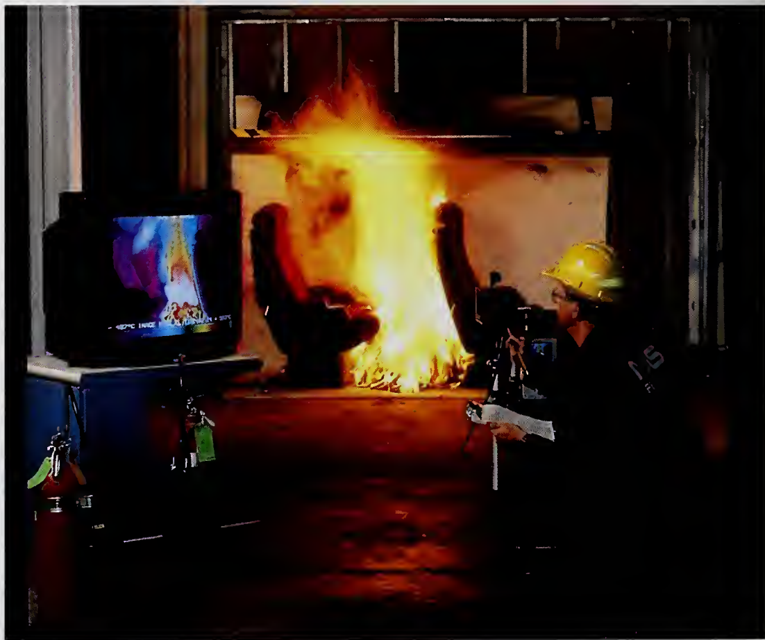
Fire protection engineer David Stroup explores the use of an infrared camera to determine details of fire spread and burning of the trash fire set near train seats
