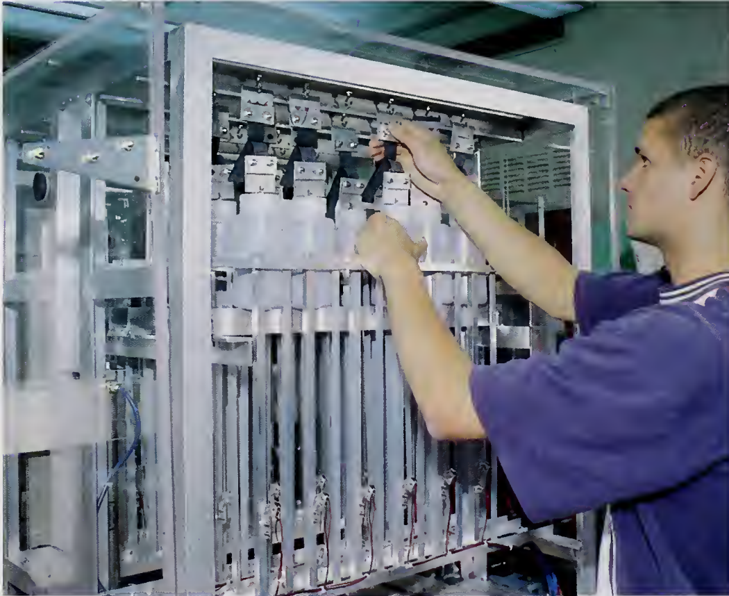
Placing tape-bonded seam specimens in the chamber prior to conducting a creep-rupture test
