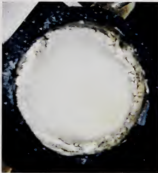
Foam-like residue of silicone with 1% silica after 50 \text{ kW/m}^2 exposure in a nitrogen atmosphere
