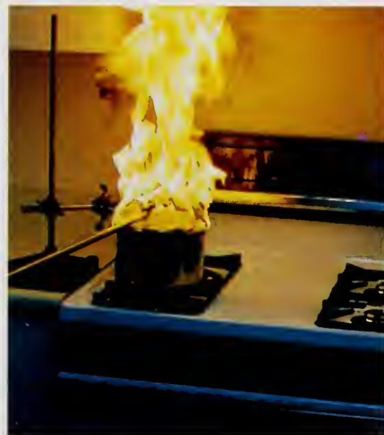
Range-top fire test
