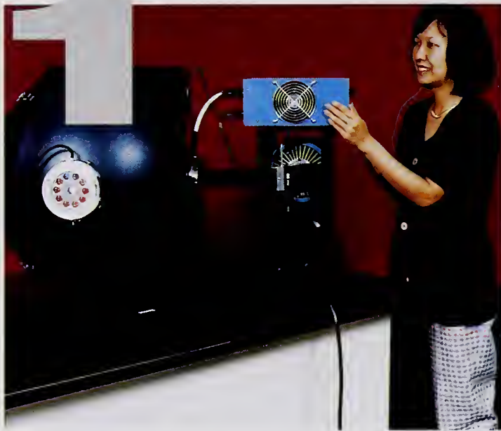
Advanced photodegradation device capable of exposing polymeric materials to a highly, spatially uniform ultraviolet radiant flux.
