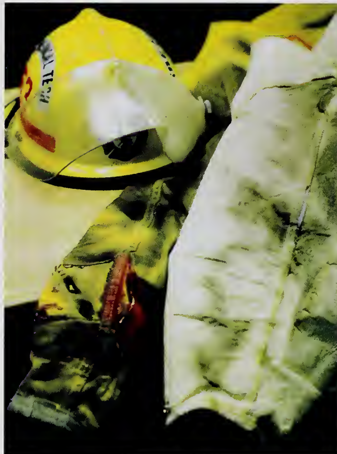
Fire Fighter turnout gear damaged during a fire that resulted in burn injuries
