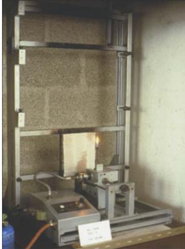
Figure 7. Vertical flammability test rig developed for the ‘Mydrin’ test.
