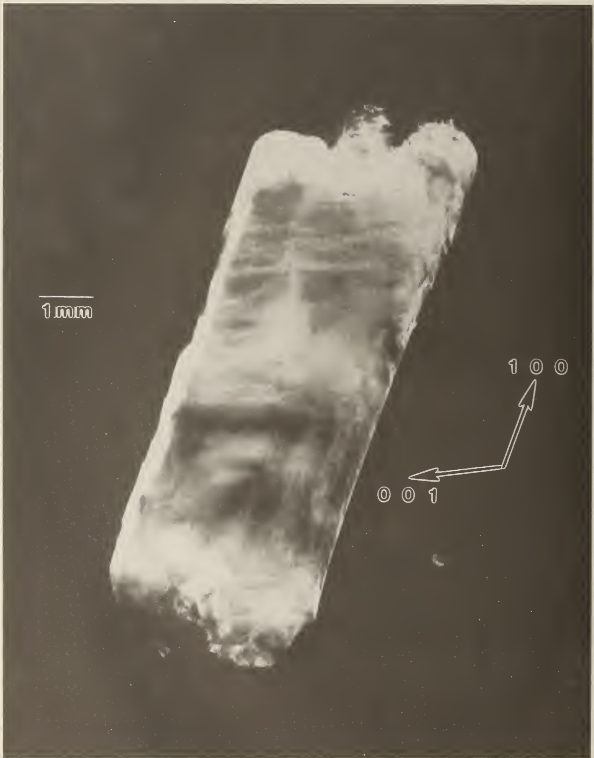
Figure 59. High-resolution (200) 10 keV diffraction image in Laue geometry from (001) surface of grain B3 of TGS crystal 120, from Spacelab III. Lighter areas diffract more strongly.
