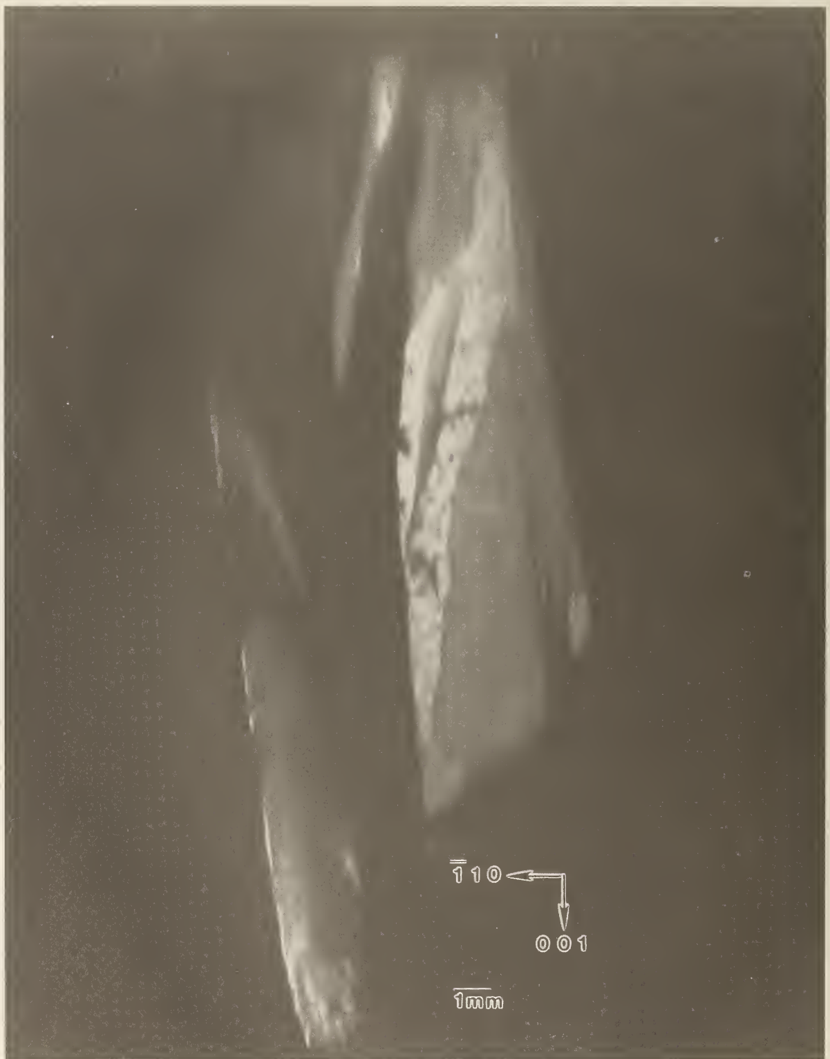
Figure 56. High-resolution (220) 8 keV diffraction image in Bragg geometry from approximately (220) surface of PbSnTe crystal \bar{1}\bar{1}\bar{1} , grown on STS 61A. The growth direction is [001]. Lighter areas diffract more strongly.
