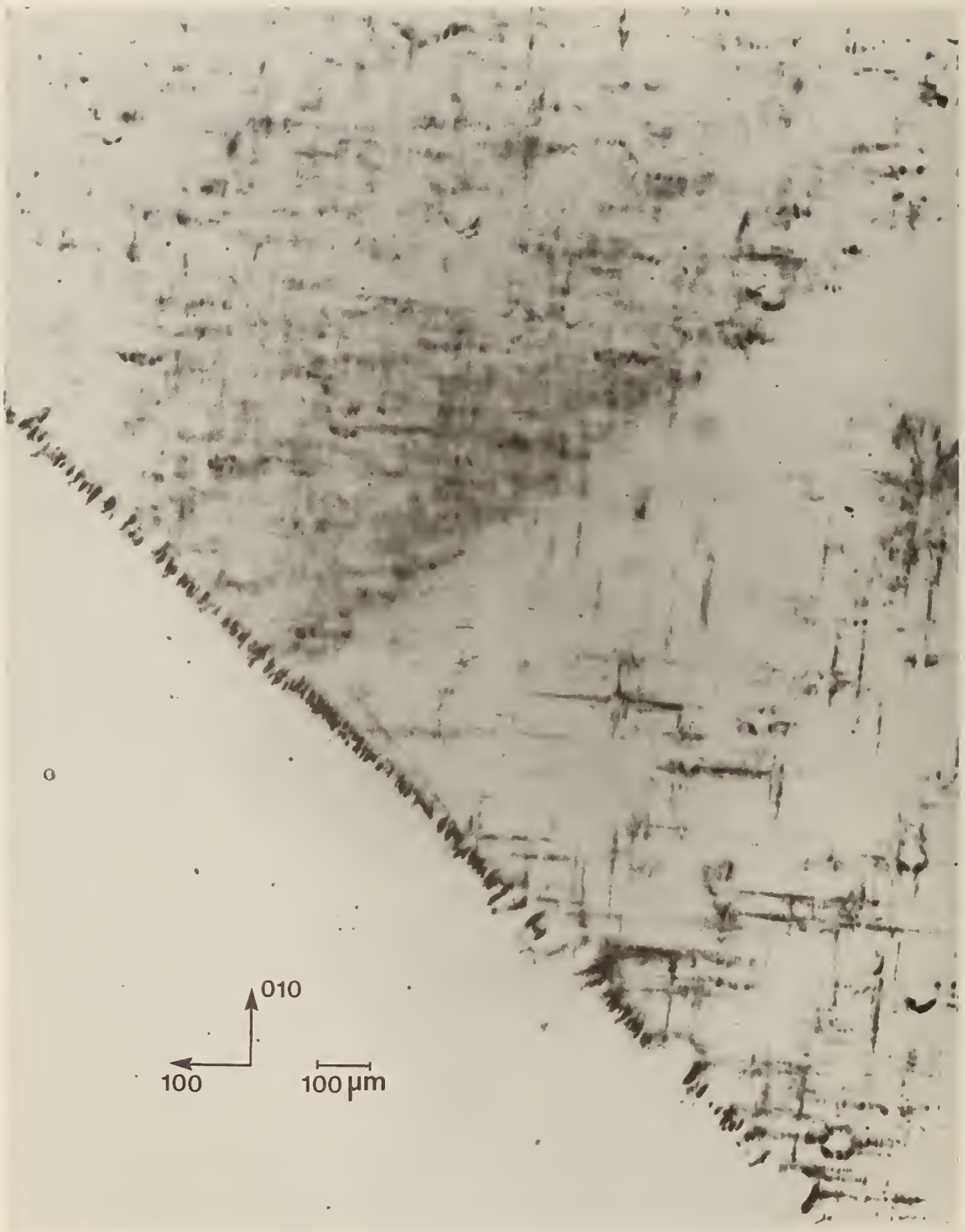
Figure 15. Enlargement of the central portion of figure 3, (0 1 10) diffraction. This image is to be compared with the same crystal region imaged in (1 1 12) diffraction, figure 7, and in (1 1 10) diffraction, figure 10. Darker areas diffract more strongly.
