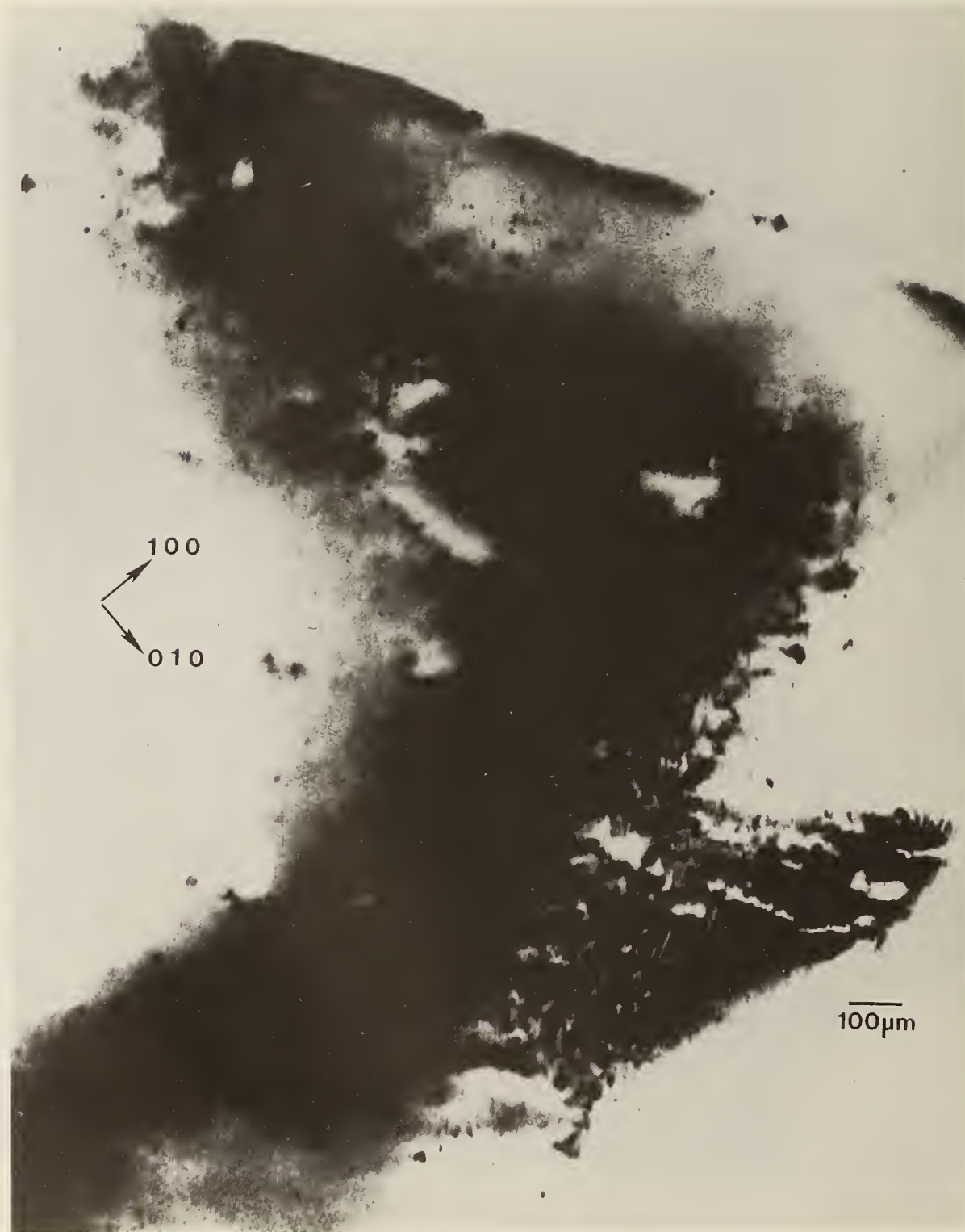
Figure 30. Enlargement of main region of figure 27, (1 1 10) diffraction. Darker areas diffract more strongly.
