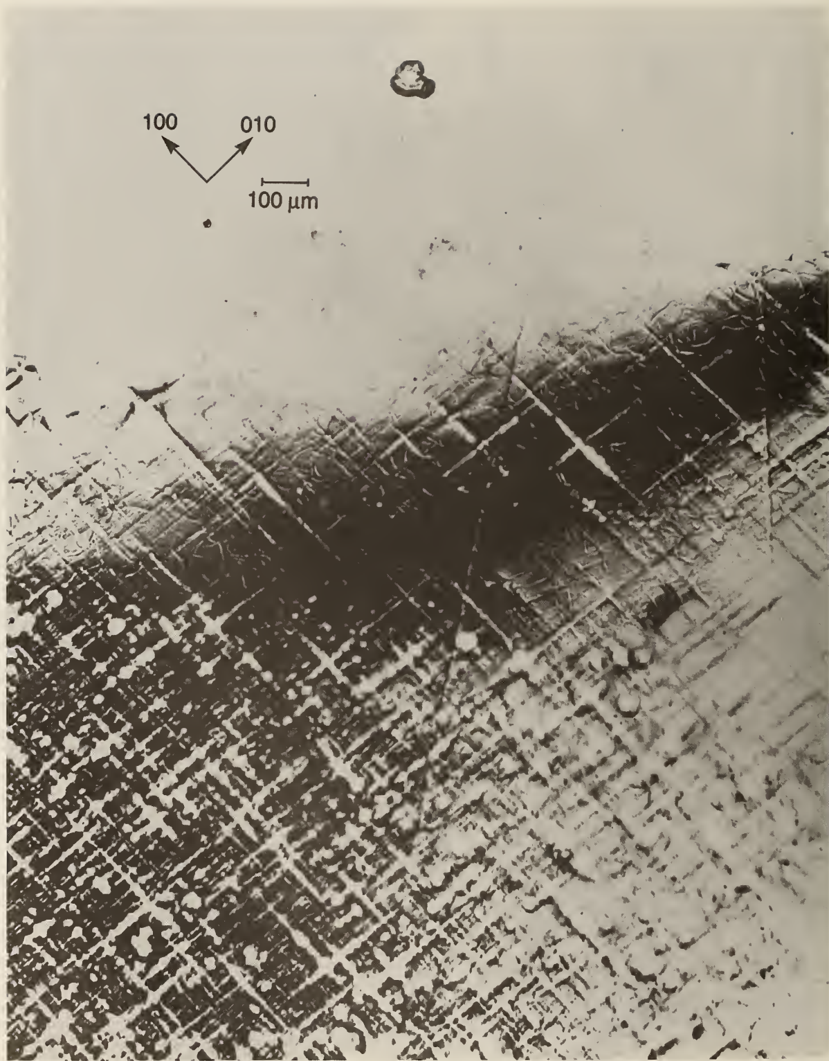
Figure 9. Enlargement of upper central portion of figure 1, (1 1 12) diffraction. Darker areas diffract more strongly.
