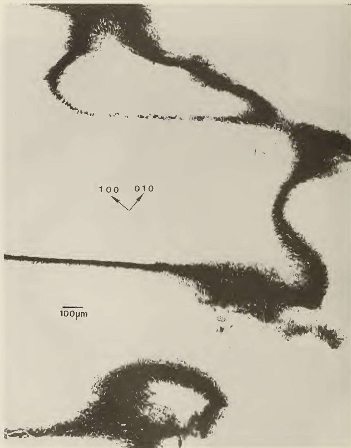
Figure 35. Enlargement of lower central portion of figure 33, (1 1 10) diffraction. Darker areas diffract more strongly.
