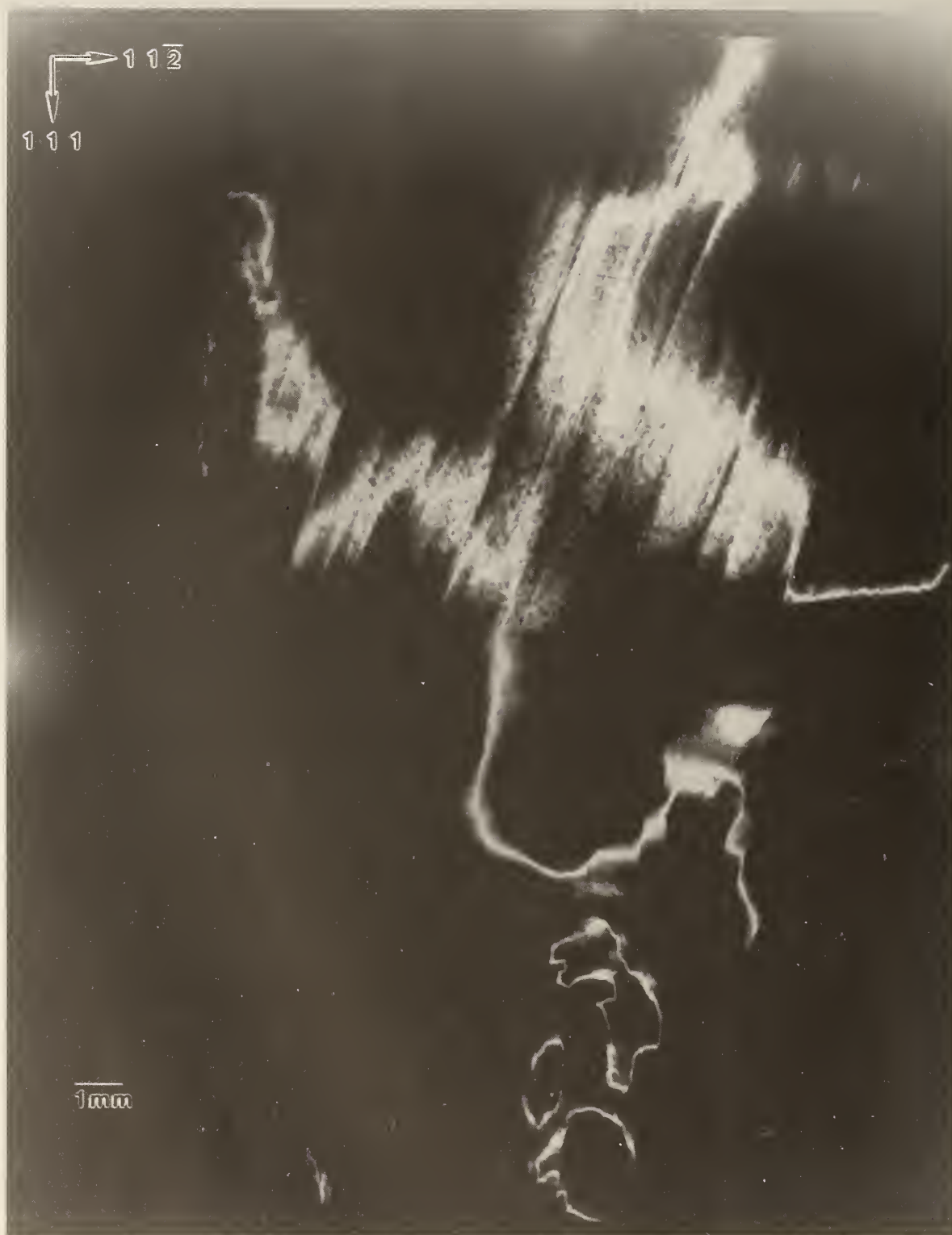
Figure 76. High-resolution (242) 10 keV diffraction image of approximately (220) surface of terrestrial GaAs crystal 119, in Bragg geometry. The growth direction is [111]. Lighter areas diffract more strongly.
