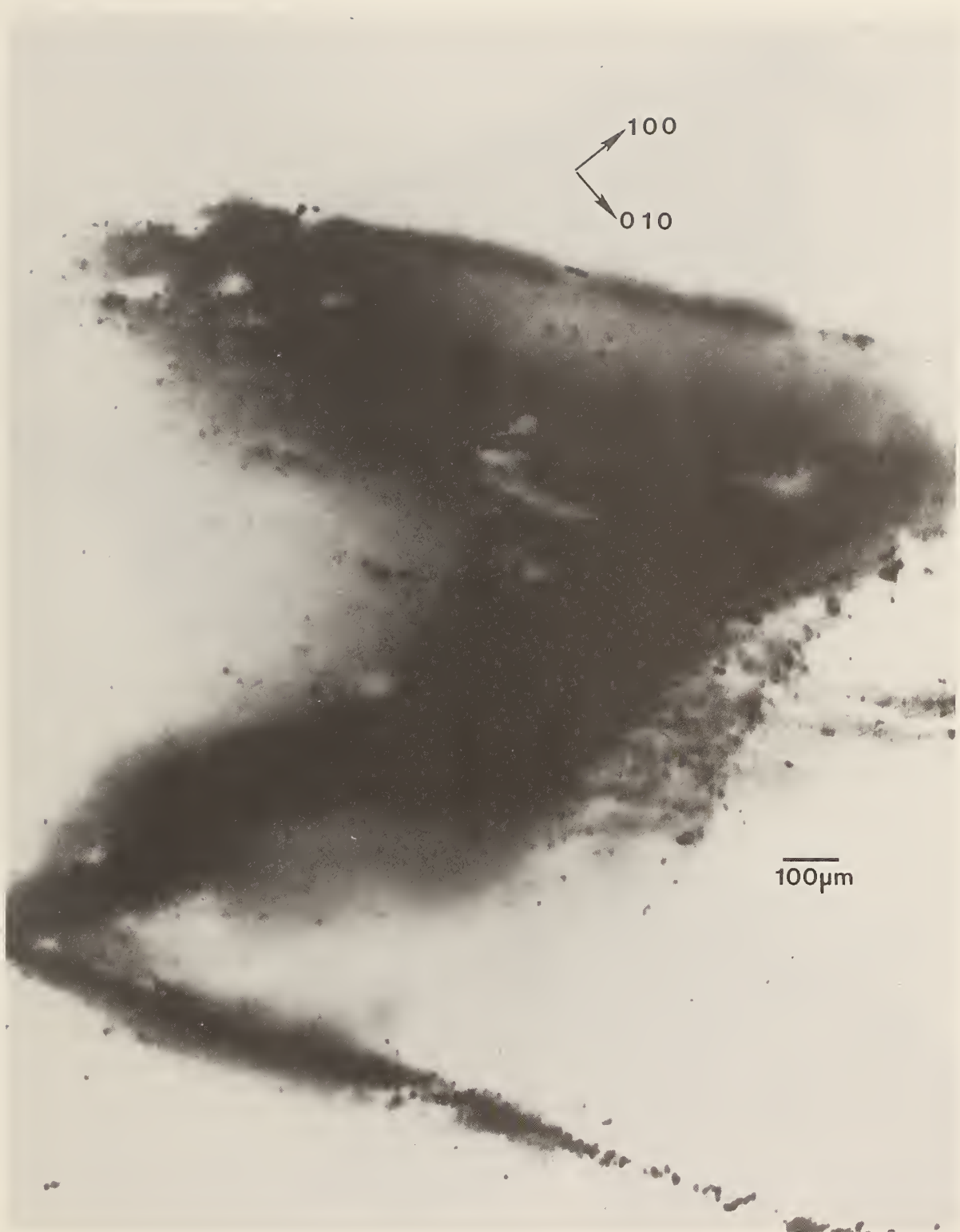
Figure 29. Enlargement of main region of figure 26, (008) diffraction. Darker areas diffract more strongly.
