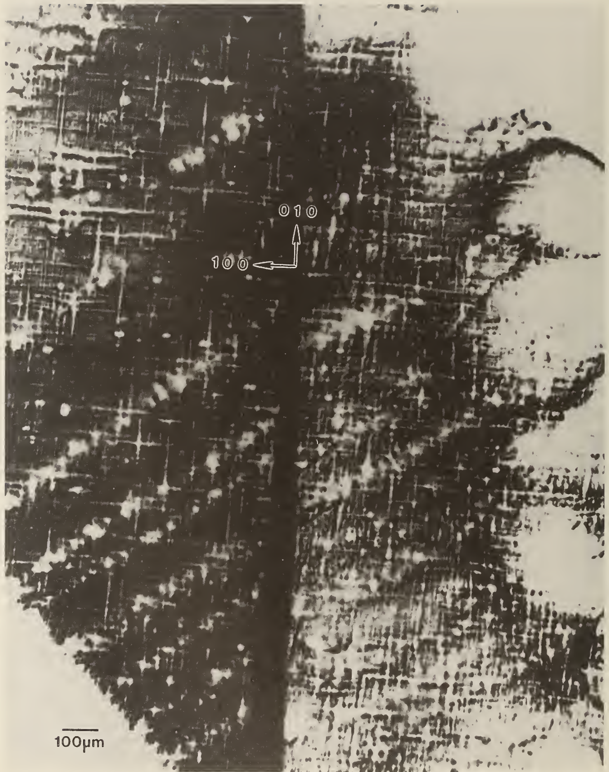
Figure 13. Enlargement of lower left-hand corner of figure 3, (0 1 10) diffraction. This image is to be compared with an overlapping crystal region imaged in (1 1 12) diffraction, figure 8, and in (1 1 10) diffraction, figure 11. Darker areas diffract more strongly.
