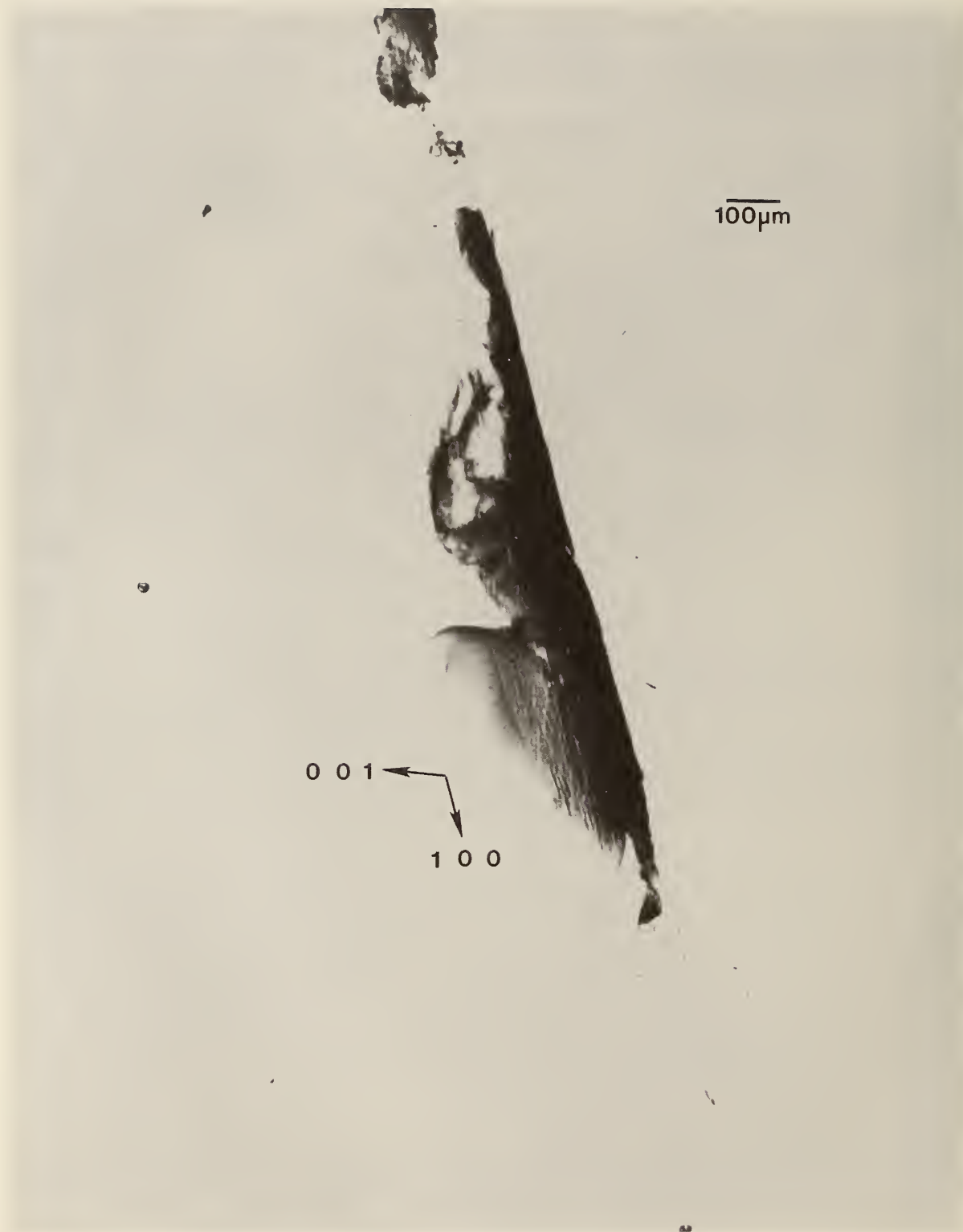
Figure 69. Enlargement of lower left-hand edge of figure 61, (200) diffraction. Darker areas diffract more strongly.
