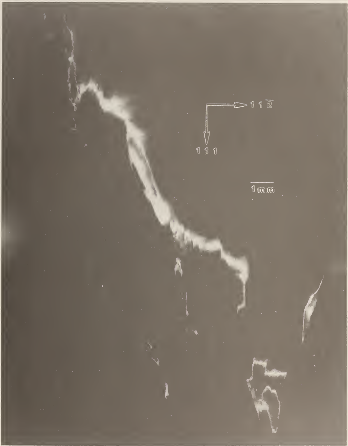
Figure 75. High-resolution (220) 8 keV diffraction image of approximately (220) surface of terrestrial GaAs crystal 119, in Bragg geometry. The angle of incidence is 3.9 arc minutes larger than in that for figure 38; the growth direction is [111]. Lighter areas diffract more strongly.
