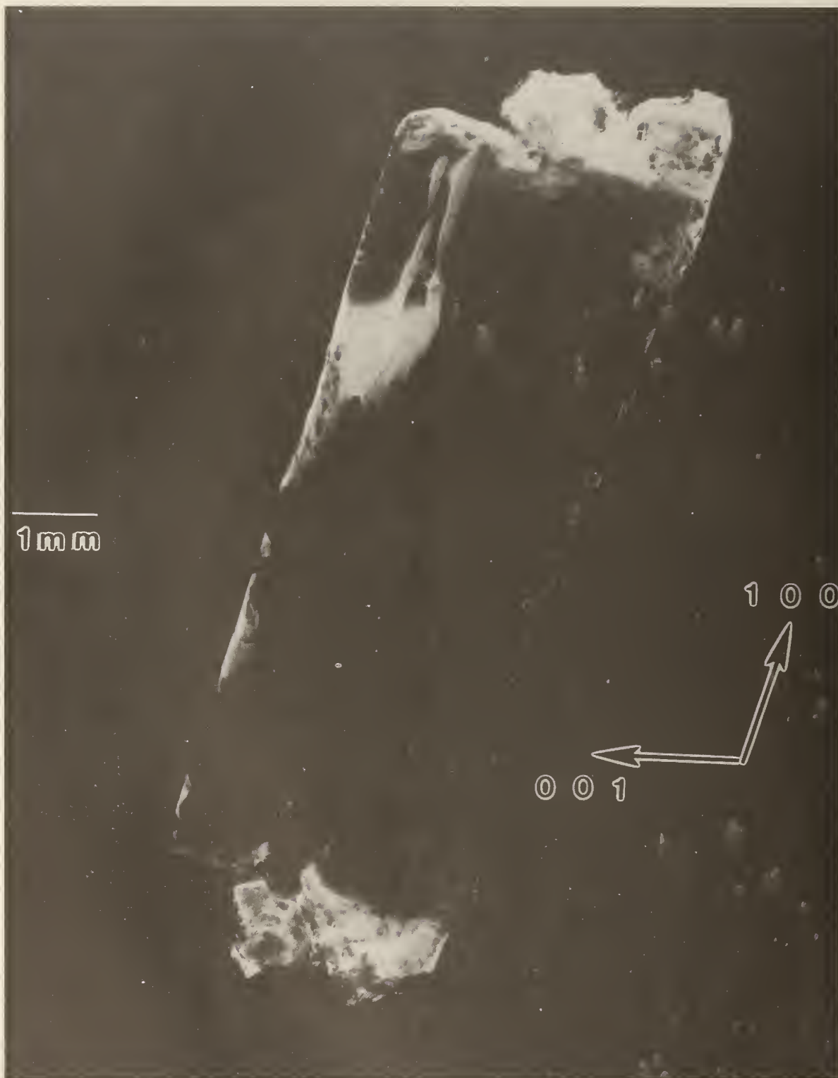
Figure 61. High-resolution (200) 10 keV diffraction image in Laue geometry from grain B1 of TGS crystal 120, from Spacelab III. Lighter areas diffract more strongly.
