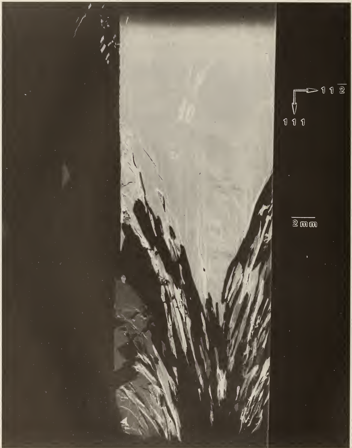
Figure 72. Low resolution (220) 8 keV diffraction image of approximately (220) surface of terrestrial GaAs crystal 119, in Bragg geometry. The sample was rocked through an angle of 4^\circ during this exposure; the growth direction is [111] . Lighter areas diffract more strongly.
