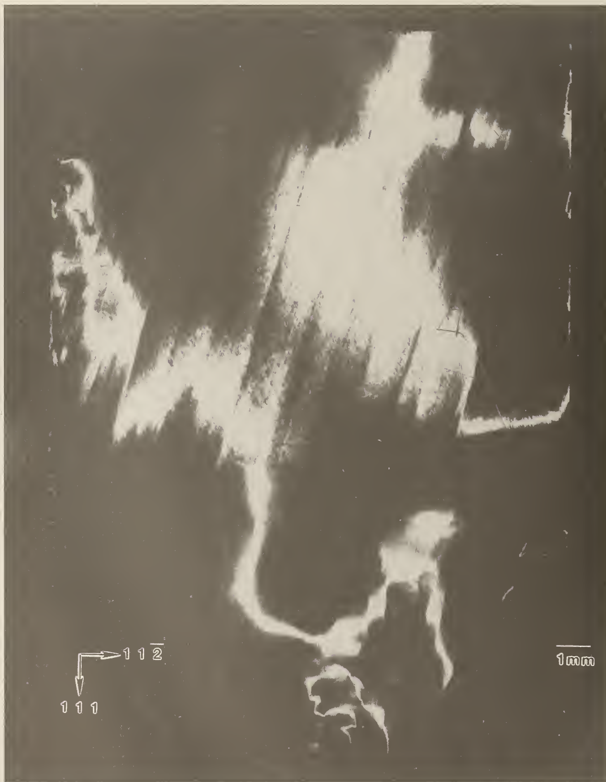
Figure 74. High-resolution (220) stationary diffraction image from approximately (220) surface of terrestrial GaAs crystal 119, in Bragg geometry. The growth direction is [111]. Lighter areas diffract more strongly.
