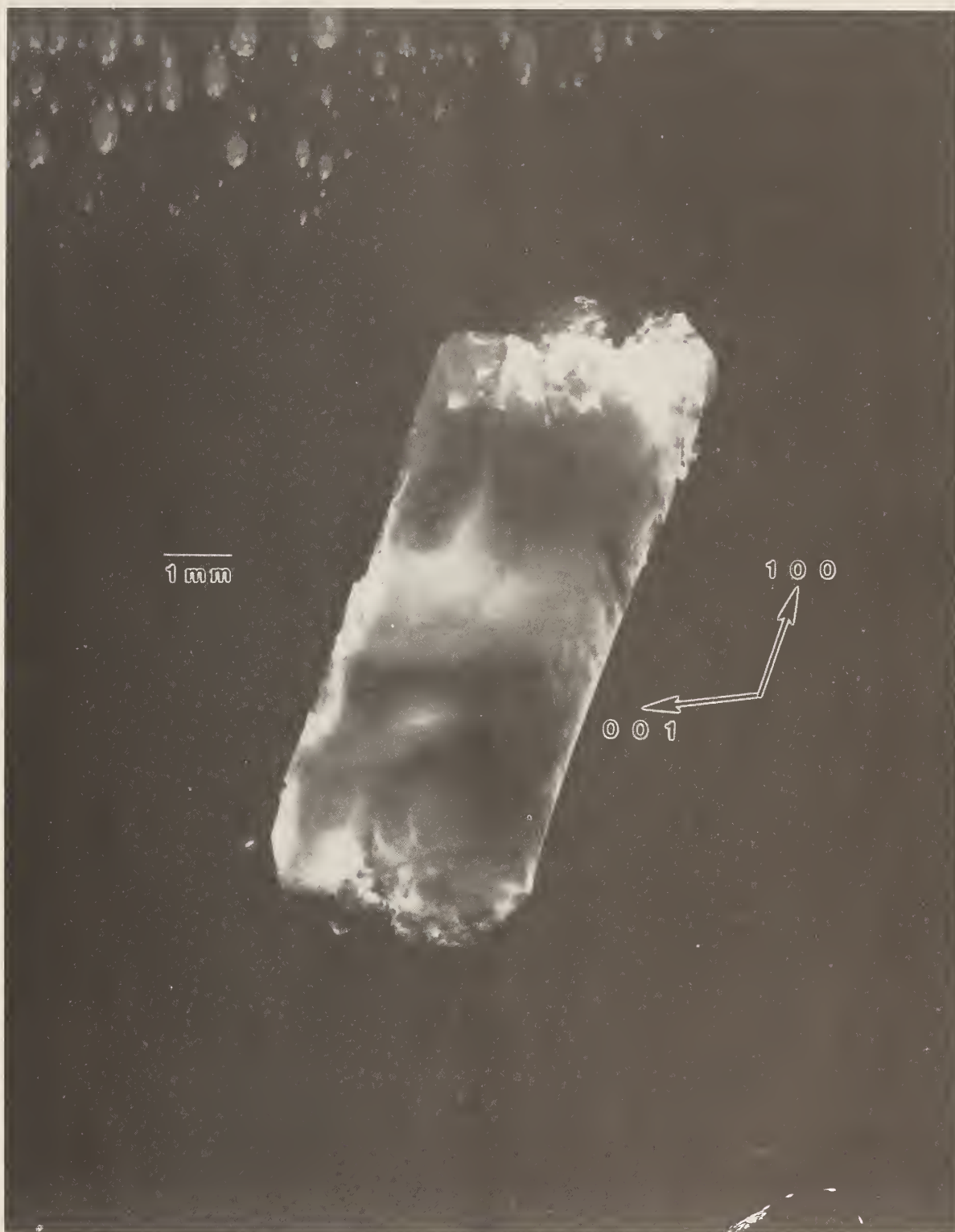
Figure 58. High-resolution (300) 10 keV diffraction image in Laue geometry from (001) surface of grain C2 of TGS crystal 120, from Spacelab III. Lighter areas diffract more strongly.
