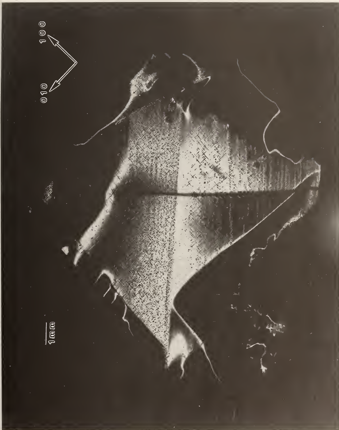
Figure 2. High-resolution (1 1 10) 8 keV diffraction image in Bragg geometry of (001) surface of terrestrial \text{HgI}_2 crystal 116, comparable to that grown on Spacelab III. Lighter areas diffract more strongly.
