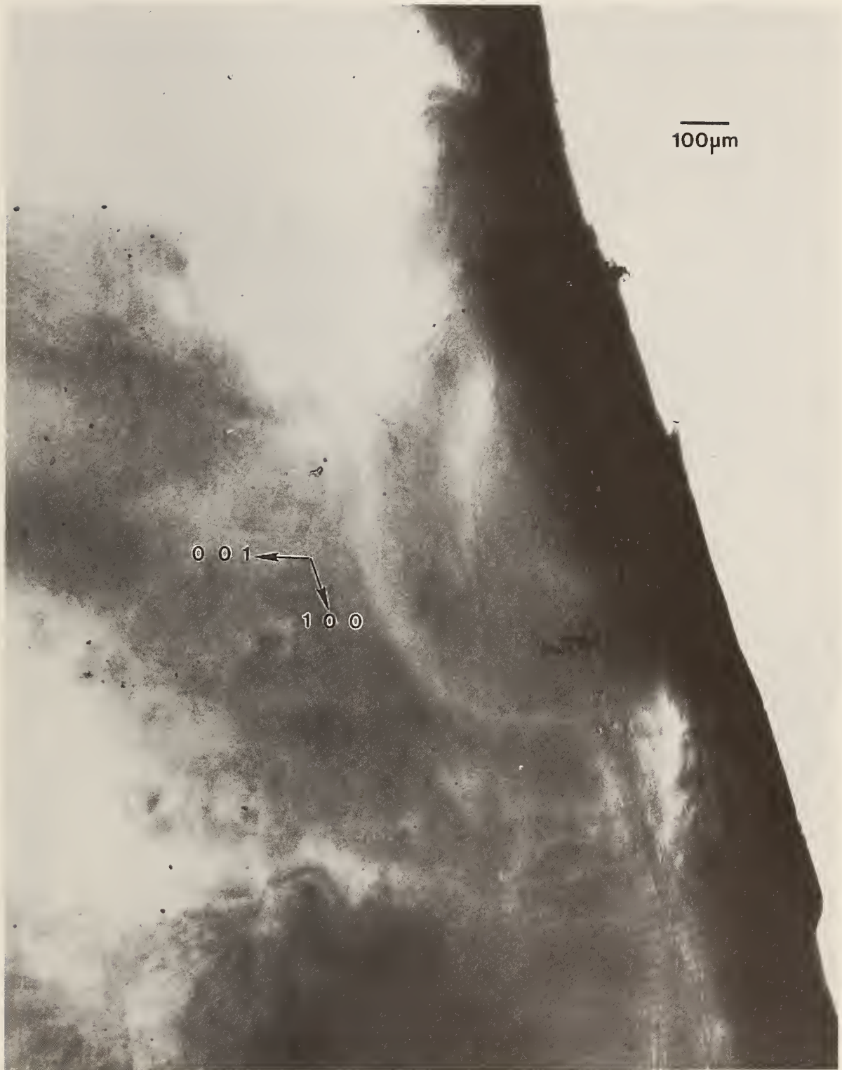
Figure 66. Enlargement of lower left-hand edge of figure 59, (200) diffraction. Darker areas diffract more strongly.
