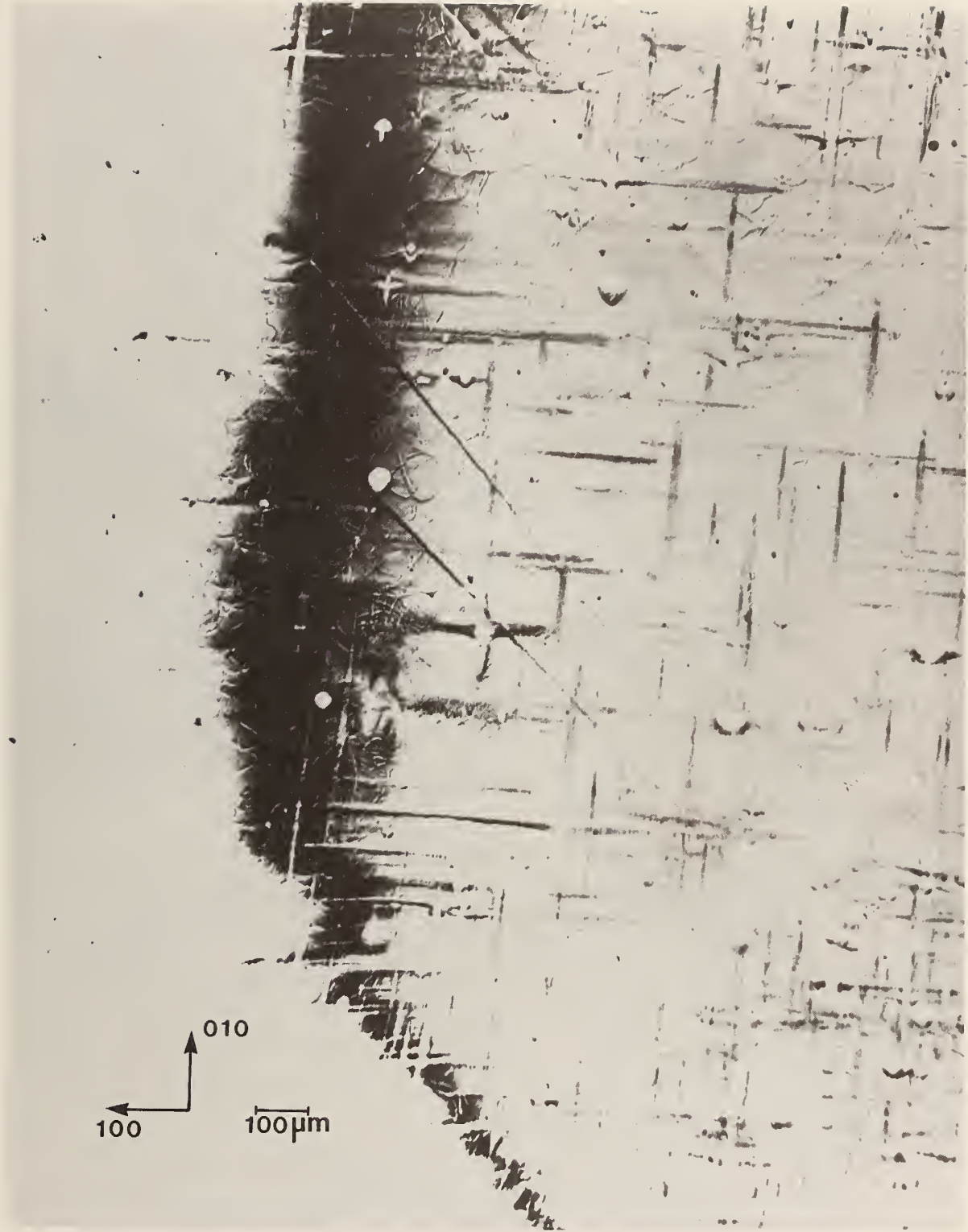
Figure 22. Enlargement of upper right central portion of figure 5, (0 1 11) diffraction. This image is to be compared with the same crystal region imaged in (0 1 10) diffraction, figure 16, and contiguous to the region imaged in (1 1 12) diffraction, figure 9, and in (1 1 10) diffraction, figure 12. Darker areas diffract more strongly.
