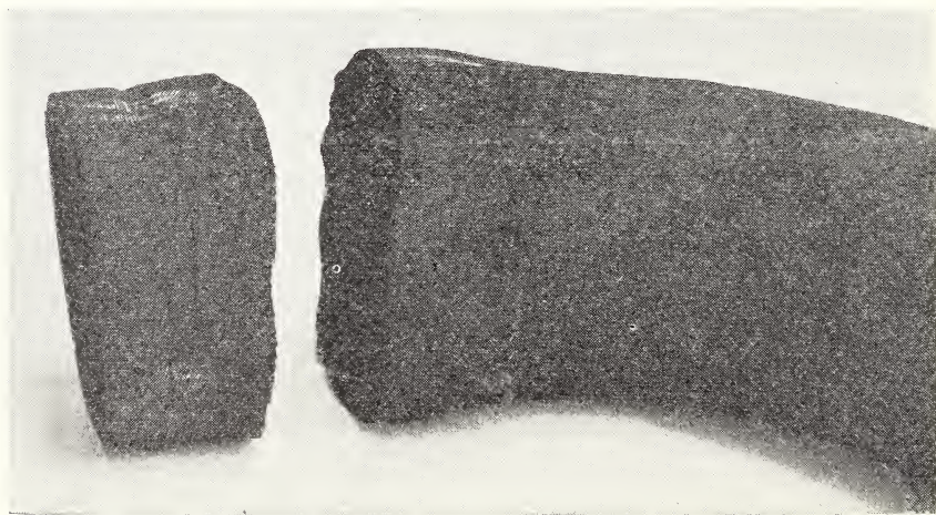
FIGURE 5. Automotive radiator hose after 7 days' use with petroleum antifreeze.
