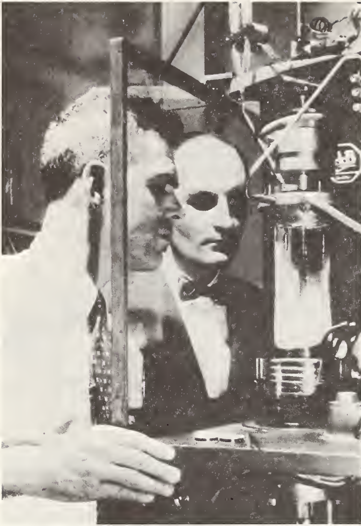
FIGURE 40. A crystal-growing apparatus of the form developed by G. K. Teal being observed by Mr. E. Buehler, who grew most of the crystals used in semiconductor development and research at Bell Laboratories for many years, and M. Sparks who fabricated the first of the good junction transistors.
