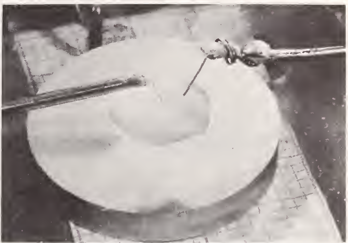
FIGURE 17. The experimental apparatus of patents 1 and 2 consisting of a point-contact passing through a drop of electrolyte with a "grid" electrode in the form of a ring (not visible in the figure) in the electrolyte.
