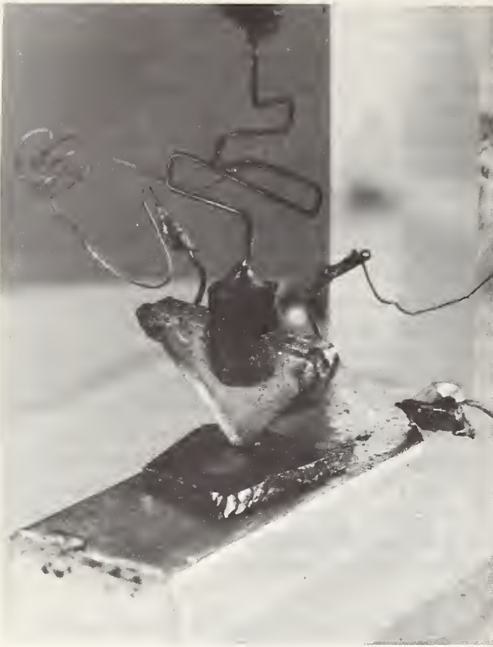
FIGURE 7. The original point-contact transistor structure comprising the plate of n-type germanium and two line-contacts of gold supported on a plastic wedge.
