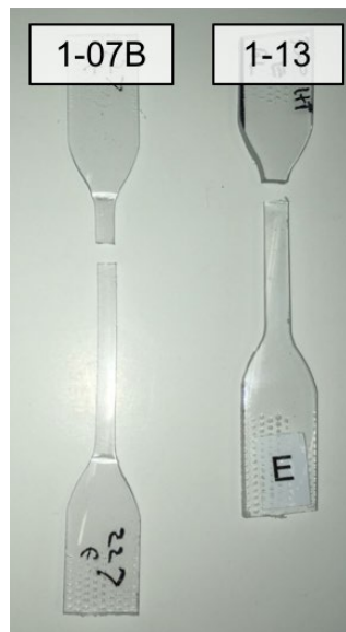
Figure 14. Representative samples of elongation following quasistatic tensile testing of unexposed facepiece sections.
