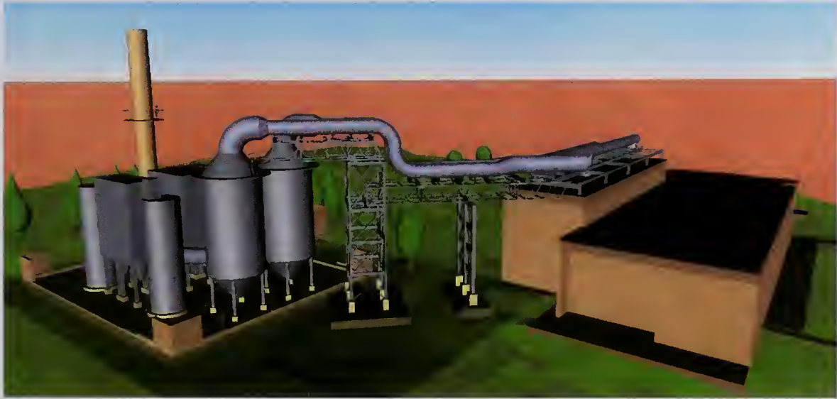
Computer generated image of emissions control system for the BFRL Fire Research Facility. This project will serve as a major field test for the LiveView framework and integrated wireless metrology systems in 2000.
