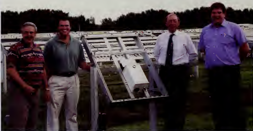
Larry Masters (President of Atlas Weathering Services Group), Jack Martin (Atlas), Larry Kaetzel (consultant), and Jonathan Martin (NIST) at Atlas' Miami exposure site standing next to a Smithsonian Institution filter-wheel solar radiometer. Four exposure sites have been equipped with this radiometer which breaks the solar ultraviolet spectrum into ten nanometer increments.
