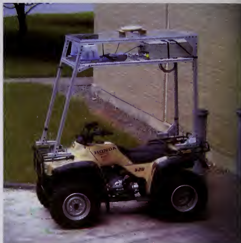
Prototype of the "strap down" construction machinery status system. The position and orientation of the vehicle are relayed to the project database in real-time.
