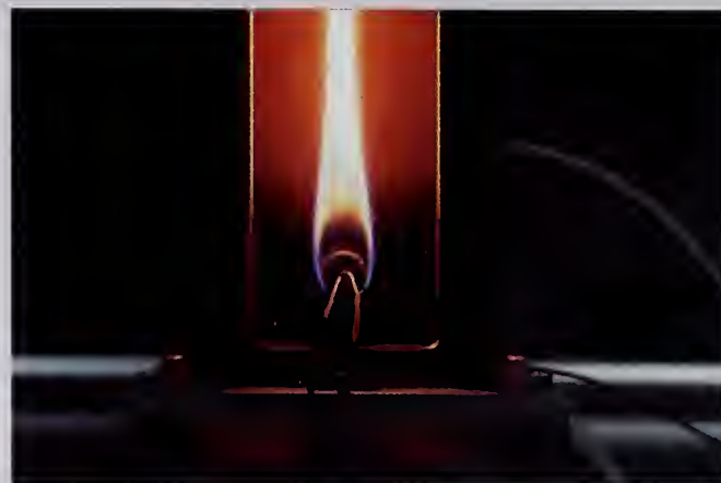
Transition from a stable enveloped flame (top) to a wake flame (right)
