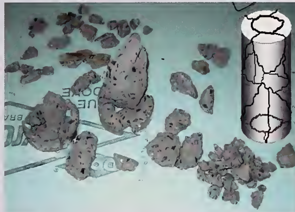
Below: Remnants of an exploded HPC cylinder and rendering of the fracture formation. The sudden, dramatic spalling failure occurs when the concrete core temperature exceeds 250°C.
