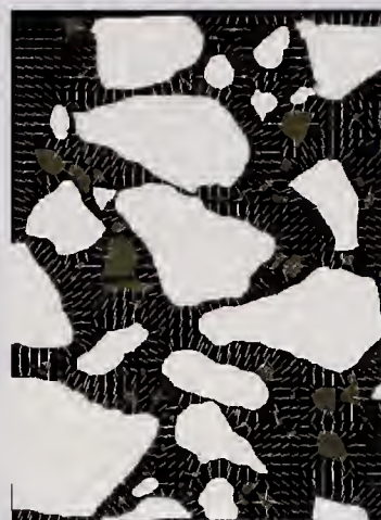
(Top) Cracking associated with both the coarse aggregate (carbonate) and chert in the coarse sand fraction. (Bottom) Crack patterns modeled by a simulated aggregate expansion show good agreement with those in the actual specimen.
