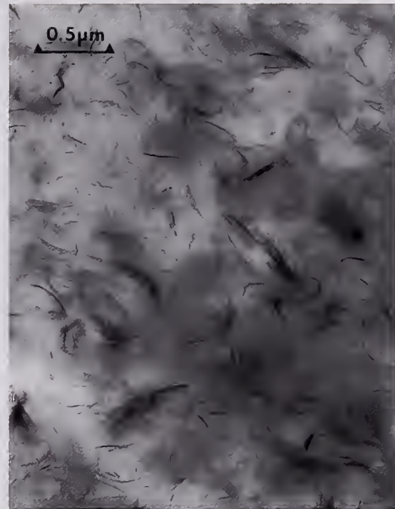
A TEM of a polypropylene-montmorillonite nanocomposite made at NIST
