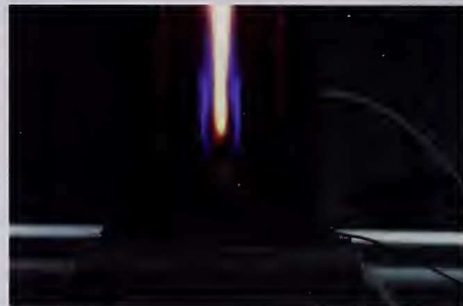
Transition from a stable enveloped flame (top) to a wake flame (right)
