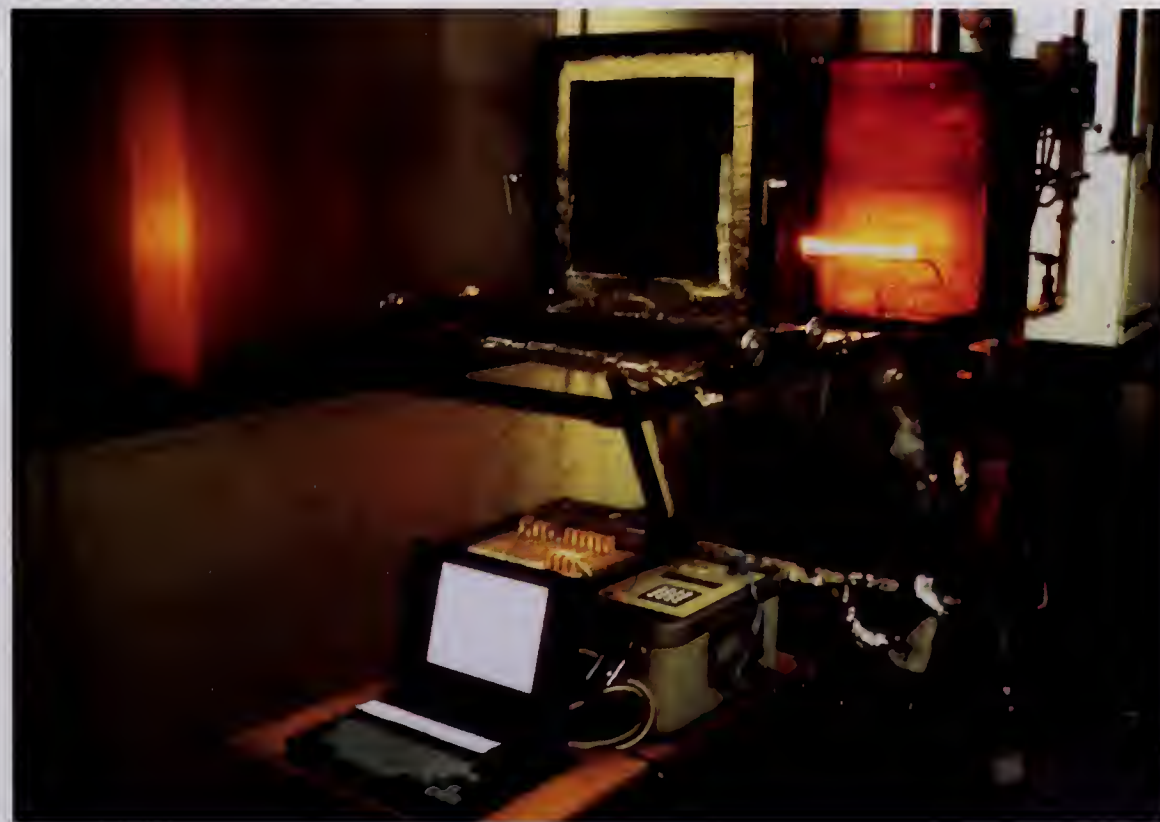
BFRL apparatus for measuring the thermal performance of fire fighter protective clothing.
