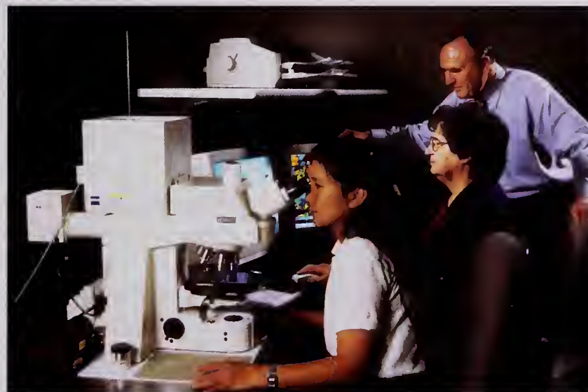
Drs. Lipin Sung, Mary McKnight and Geoffrey Erobudorff view a confocal microscopic image of an optical slice through the thickness of a coating. The confocal microscope has an optical resolution down to 200 nm and is a major research tool in assessing the microstructural properties of coatings.
