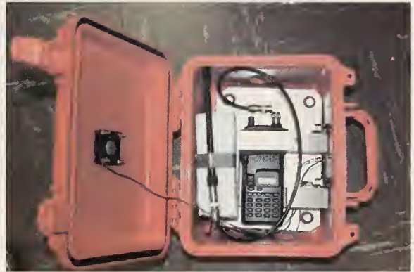
Figure 5. Typical transmitters used for the lower four frequency bands.
