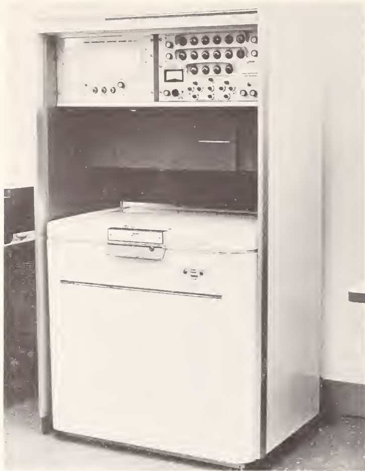
Figure 5. Liquid scintillation counter used for determining carbon-14 and tritium.
