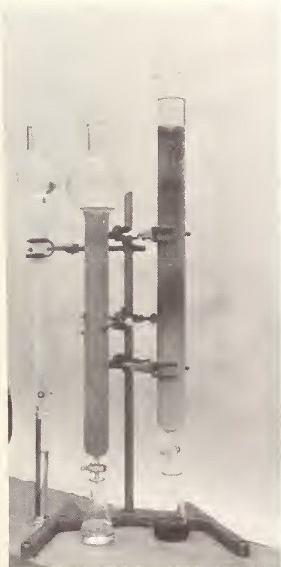
Figure 2. Column separation of oxidation products of pyrene.
