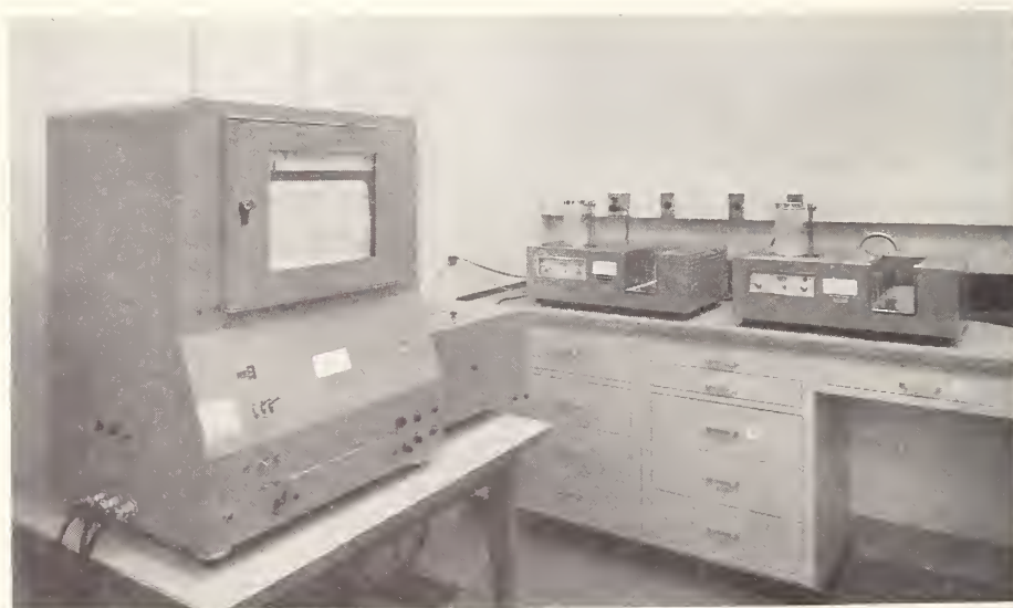
Figure 1. Portion of equipment used in measurement of ultraviolet, visible, and infrared spectra.
