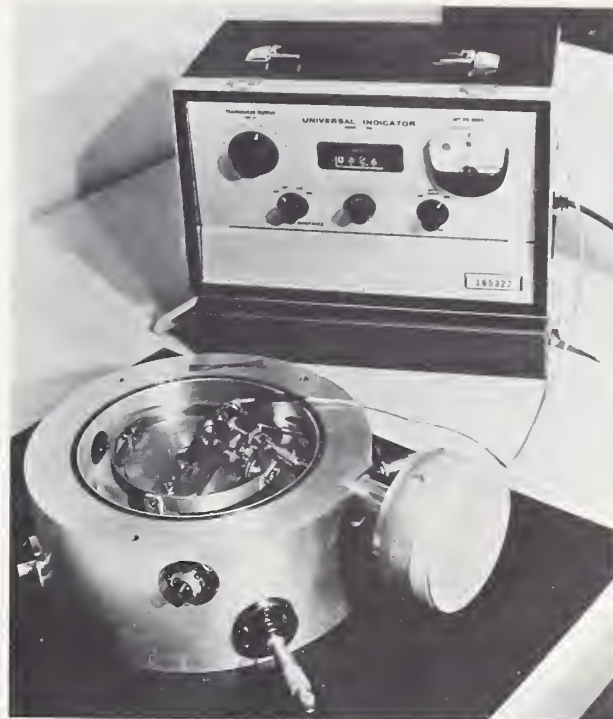
FIGURE 19a. Loading device mounted in Kossel camera. Readout unit is at rear.
