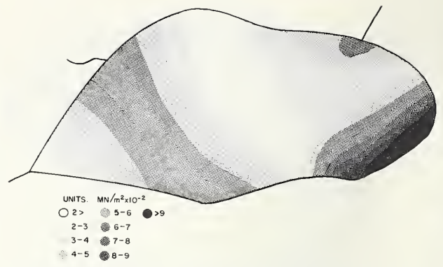
FIGURE 35a. Total stored elastic energy, W , in \text{MN/m}^2 \times 10^{-2} , as a function of position in grain, Level I.
