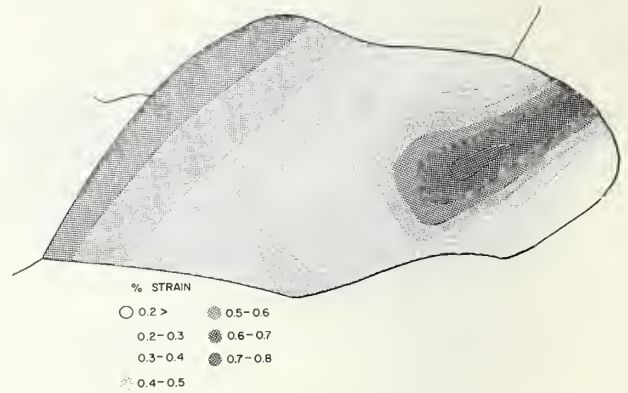
FIGURE 39b. Absolute value of the maximum shear strain in the (112) plane as a function of position in grain, Level II.
