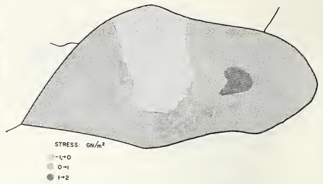
FIGURE 30b. Maximum principal stress in GN/m 2 as a function of position in grain, Level II.
