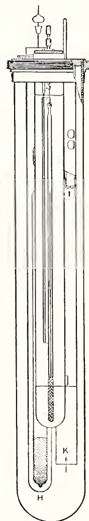
FIGURE 2. Densimeter tube H in inner water bath, one-fourth size (Osborne).
