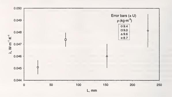
Figure 11 - Thermal conductivity measurements of Fibrous-Glass Blanket NIST CTS as a function of Thickness
