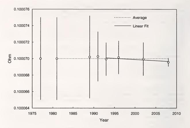
Figure 8 – Control chart for 0.1  $\Omega$  standard resistor, S/N 21736
