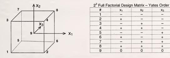
Figure 9 - Full-factorial experimental design for 3 factors, 2 levels
