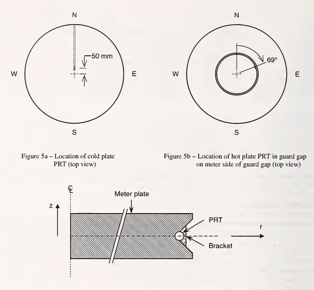
Figure 5c – Cross-section view of PRT in guard gap (guard plate not shown)
