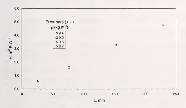
Figure 13 – Thermal resistance measurements of Fibrous-Glass Blanket NIST CTS ( $T_m$  of 297 K,  $\Delta T$  of 22.2 K)
