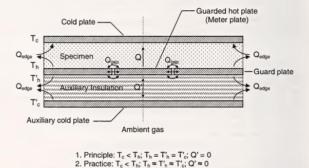
Figure 2 - Guarded-hot-plate schematic, single-sided mode of operation - heat flow up
