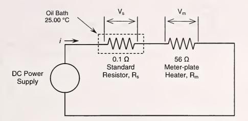
Figure 4 - Electrical schematic for meter-plate power measurement
