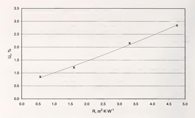
Figure 14 – Relative expanded uncertainties (k=2) versus thermal resistance of Fibrous-Glass Blanket NIST CTS
