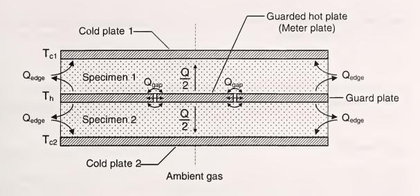
1. Principle:  $T_c < T_h$ ;  $T_{c1} = T_{c2} = T_c$ 2. Practice:  $T_c < T_h$ ;  $T_{c1} \approx T_{c2} \approx T_c$
