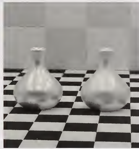
Vases rendered with two different metallic-flake pigmented coatings. The vase on the left is coated with a material having larger flakes than the one on the right and appears more specular, consistent with reflectance measurements.
