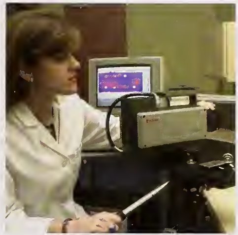
Ms. Monica Starnes using an infrared camera to assess the condition of FRP laminates bonded to concrete.
