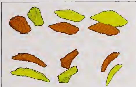
Six views, from various rotation angles, of a real aggregate particle taken from an x-ray tomographic image (orange), and the same particle, re-created using spherical harmonic analysis (yellow). The mathematical analysis correctly captures the real three-dimensional shape of the irregular aggregate particle.
