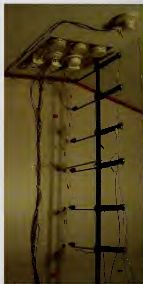
Instrumentation for smoke alarm tests in a manufactured home.
