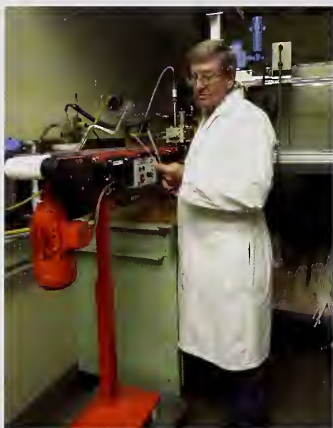
Computer-controlled gravimetric-fed twin-screw extruder used to optimize the extrusion of gradient samples with continuously varying concentrations of additives.
