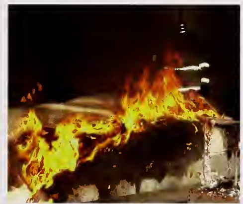
Bed fire about two minutes after ignition with a match sized flame.
