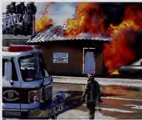
Phoenix Fire Department burn instrumented single family home for training video.
