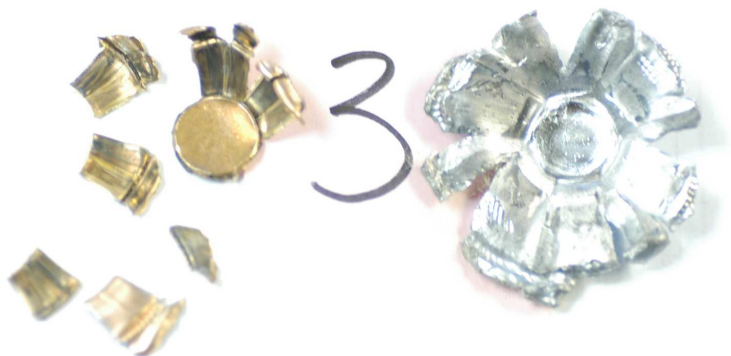
Figure 5.7: Photograph of shattered bullet removed from armor.
