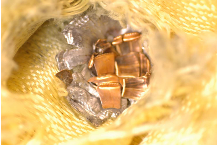
Figure 5.6: Photograph of de-constructed armor with shattered bullet inside.
