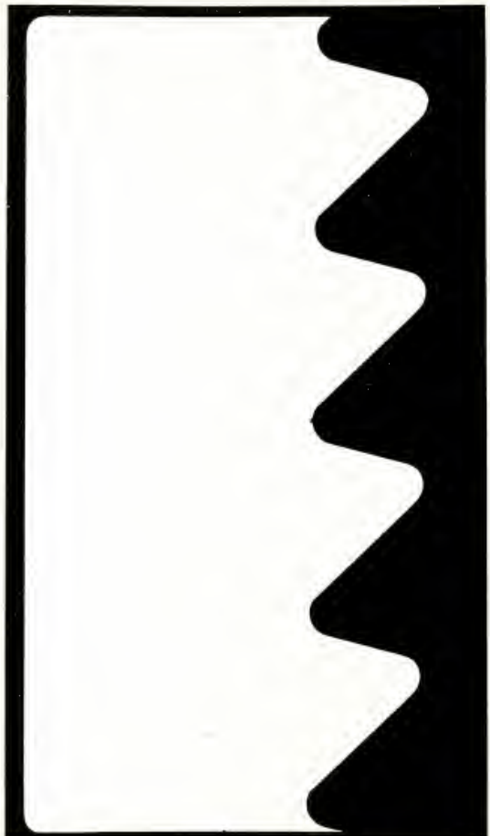
Figure 10b. Thread profile of undamaged threads of blade retention nut. X 7
