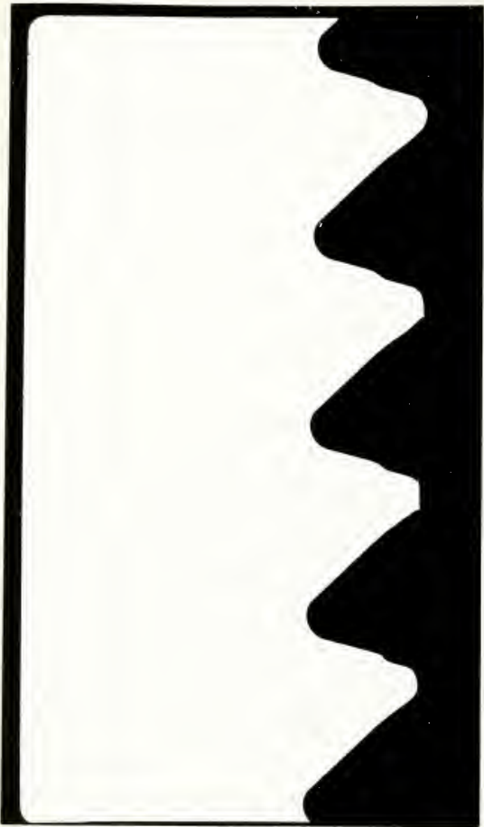
Figure 10a. Thread profile of damaged threads of blade retention nut. X 7
