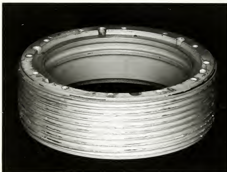
Figure 2. Blade retention nut from blade socket No. 2 as received. X 2/3
