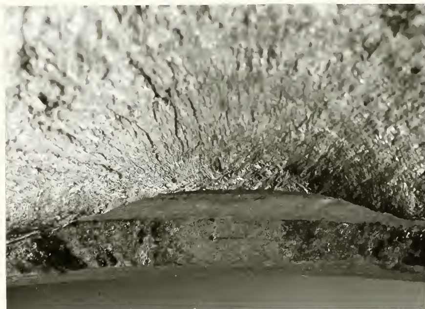
Figure 4. Origin of fatigue crack in failed hub socket, No. 2. X 10
