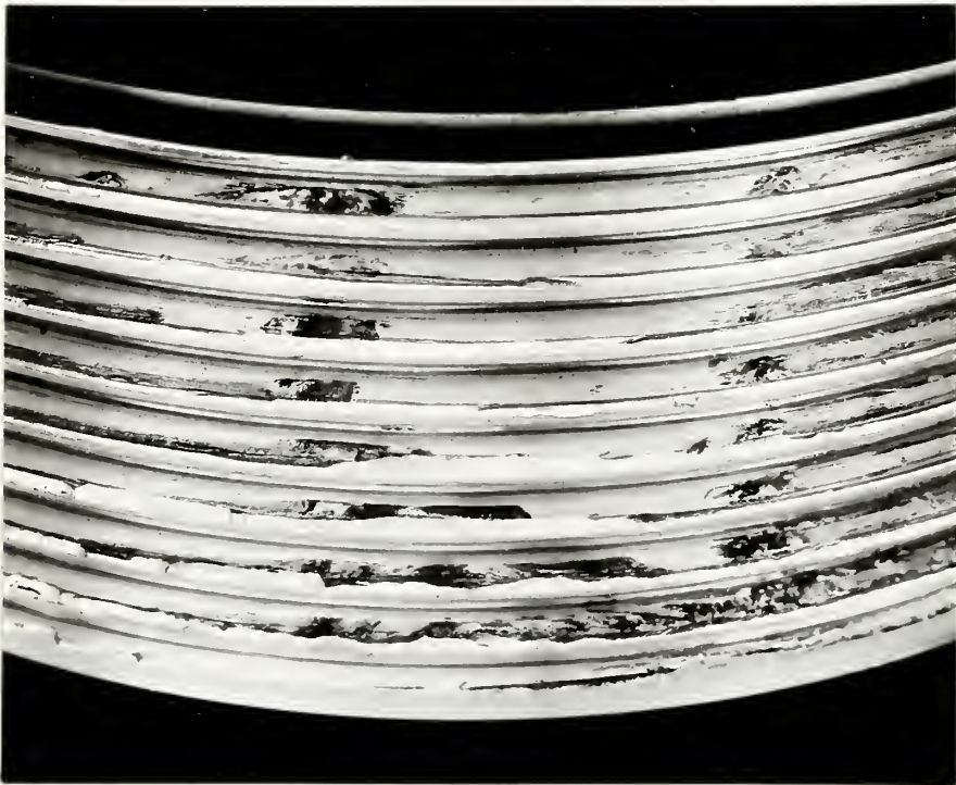
Figure 9. Threads of blade retention nut showing fretting. X 2
