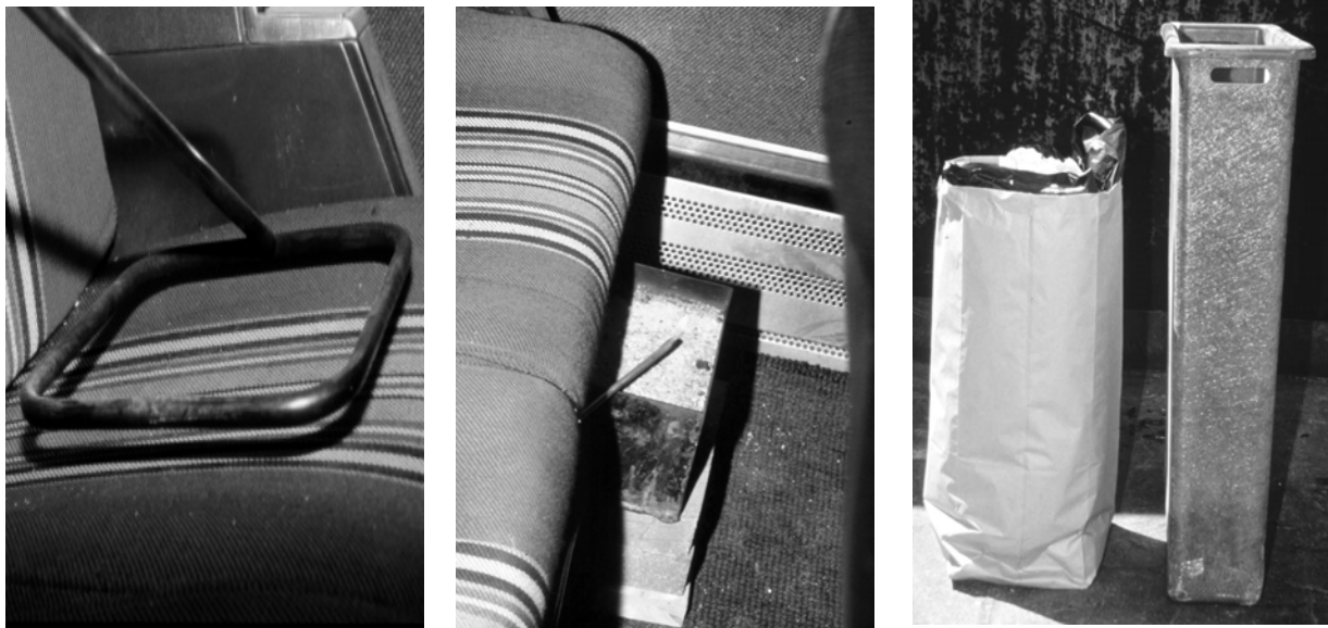
(a) TB 133 gas burner
