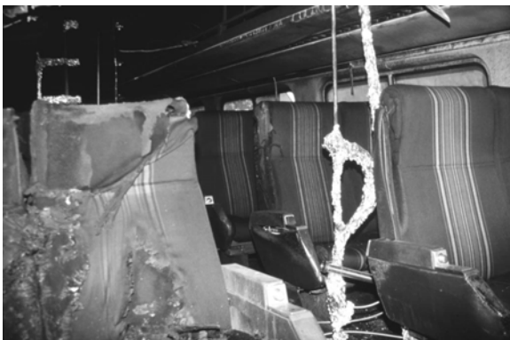
(a) Fire spread to front seat area
