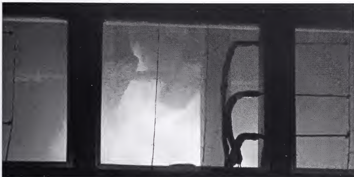
Figure 9–20. Flame impingement on trusses and bar during Test 6.
