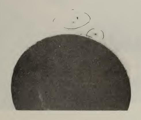
Figure 5. Typical pinholing near drain of restoration coatings
