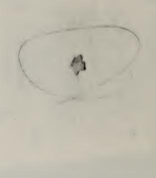
Figure 4. Typical delaminated blister of restoration coatings
