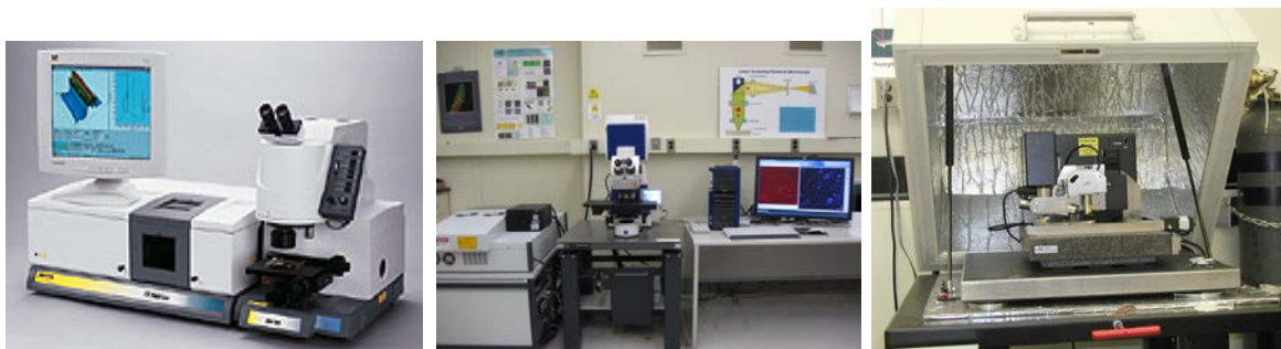
Figure 6. Photos of FTIR spectrometer, Confocal microscope and atomic force microscope (from left to right) at NIST Engineering Laboratory to be used for PV polymeric materials studies.
