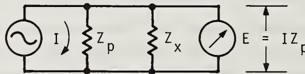
Figure 3-15. Measurement of large impedances using constant voltage generator
