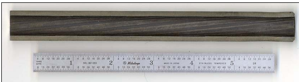
Figure 4. Stellite 21 liner removed from the first M2 machine gun barrel.
