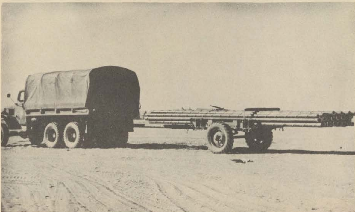
Figure 42. Two-wheeled ponton dolly loaded and hitched to a 2½-ton, 6 by 6 truck.
