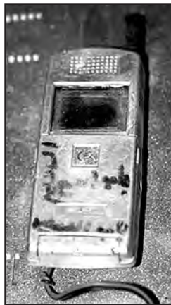
Figure 128. The growing sophistication of terrorists became evident in the wide variety of electronic devices, including this cell phone, used to detonate IEDs.
