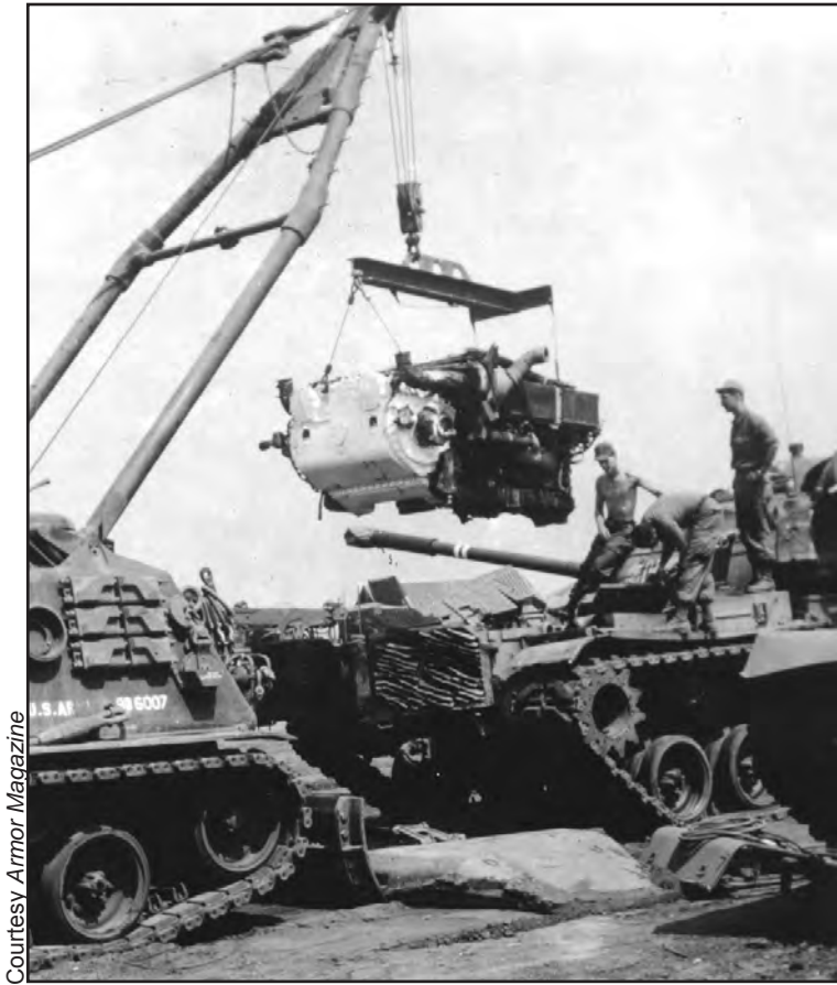
Figure 65. Replacing the M48's engine in the field.
