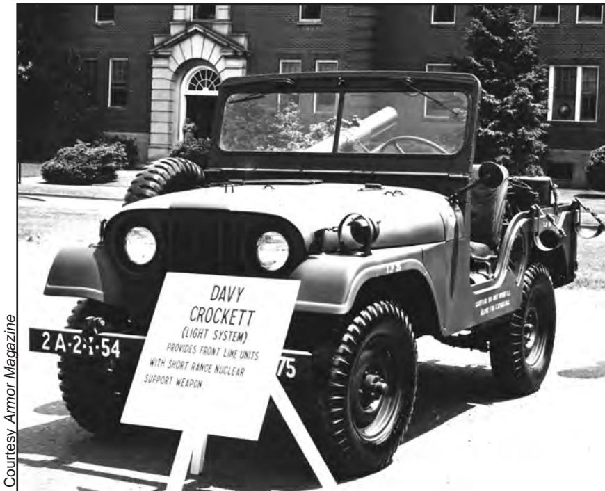
Figure 44. Light mobile Davy Crockett system to provide nuclear capability to forward units.
