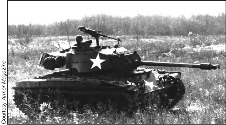
Figure 36. The M41 Light Tank (Walker bulldog) fielded to replace the M24 (Chaffee) and cope with more heavily armed and armored Soviet combat vehicles.
