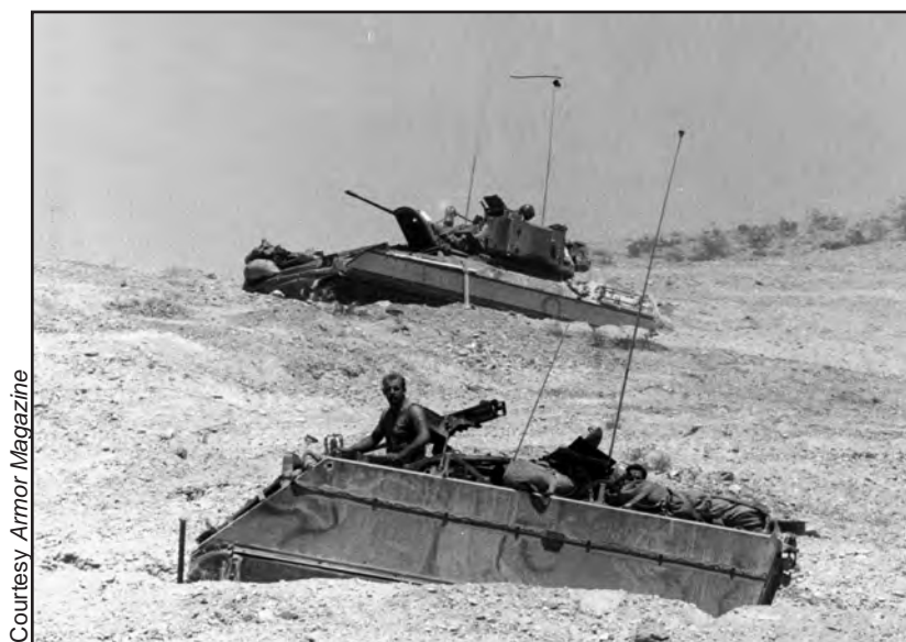
Figure 86. A Bradley Fighting Vehicle and an M113 occupy battle positions at the NTC.
