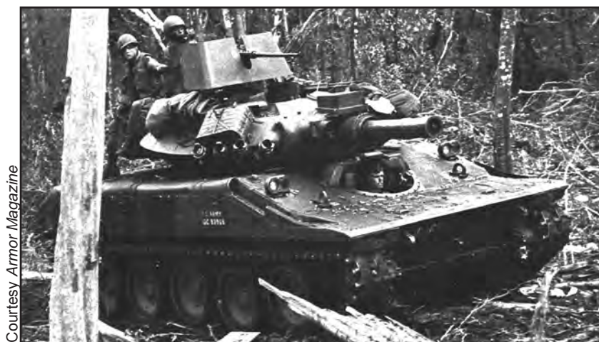
Figure 74. Sheridan with added protection for the tank commander against small arms fire and snipers.
