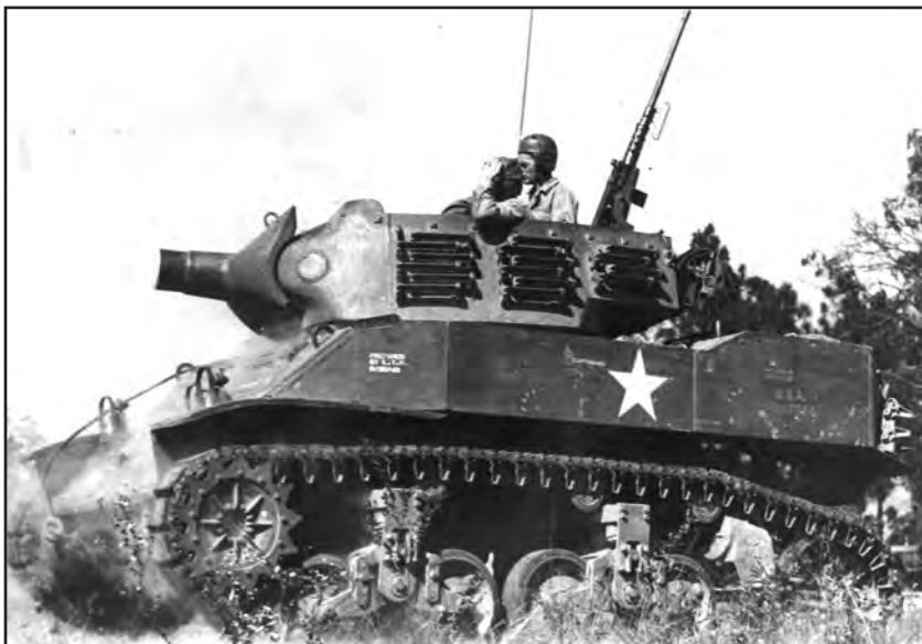
Figure 25. The M8 Howitzer Motor Carriage, which provided fire support for the mechanized cavalry.
