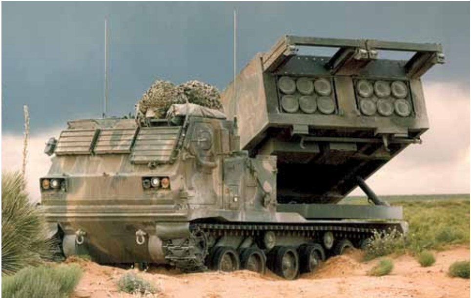
A Multiple Launch Rocket System (MLRS), capable of hitting targets at three hundred kilometers if firing the ATACMS missile
