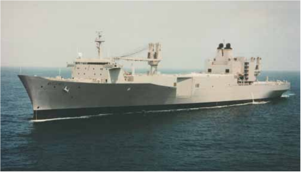
A roll-on/roll-off (RO/RO) ship sped maritime transportation of vehicles.
