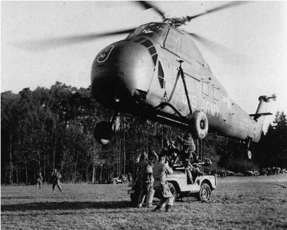
Soldiers of the 11th Airborne Division attach a ¼-ton jeep with recoilless rifle to an H-34 helicopter for air assault during Exercise SABRE HAWK.
