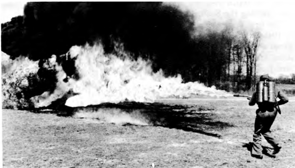
OPERATOR FIRING A PORTABLE FLAME THROWER E1R1 at a concrete fortification during a test of the weapon.
