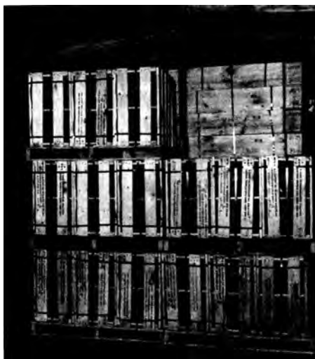
BOXED CANS OF DECONTAMINATING SOLUTION stacked on pallets, wooden platforms built to leave clearance underneath for the forks of the fork-lift truck.
