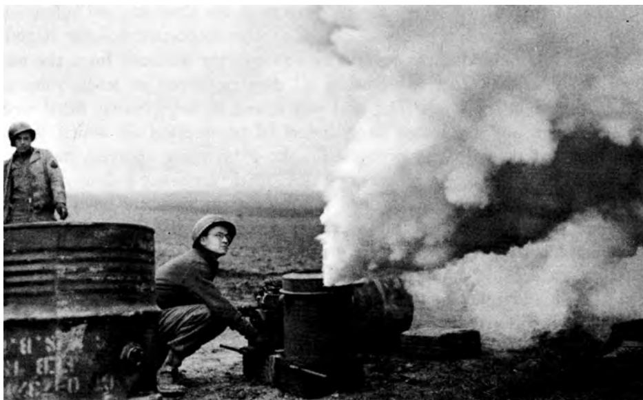
MECHANICAL SMOKE GENERATOR M2 (50-GALLON), one of many used to screen a heavy ponton bridge over the Rhine River, Germany.
