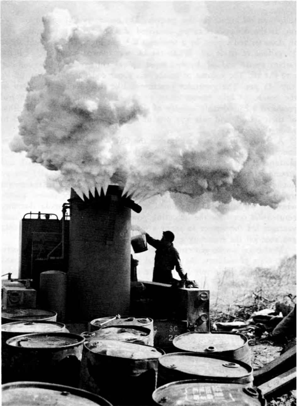
MECHANICAL SMOKE GENERATOR M1 (100-GALLON) pouring out smoke screen to conceal Fifth Army operations from the Germans, Anzio area, Italy, March 1944.
