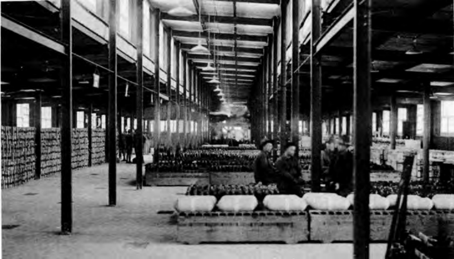
PLANT AT EDGEWOOD ARSENAL where filled shells were classified, tested for leaks, painted, and boxed for shipment. Livens drums, foreground, were painted with two white stripes to indicate they were filled with phosgene.
