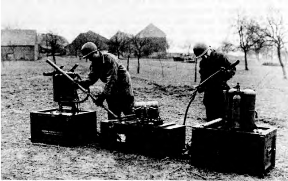
AMERICAN AND GERMAN PORTABLE FLAME THROWERS. U.S. flame thrower M2-2, left; German 1942 model, right.
