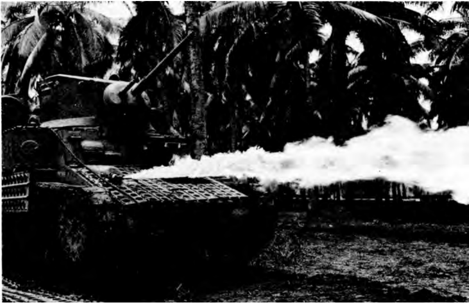
M3A1 LIGHT TANK EQUIPPED WITH FLAME GUN firing during a demonstration, New Zealand, October 1943.
