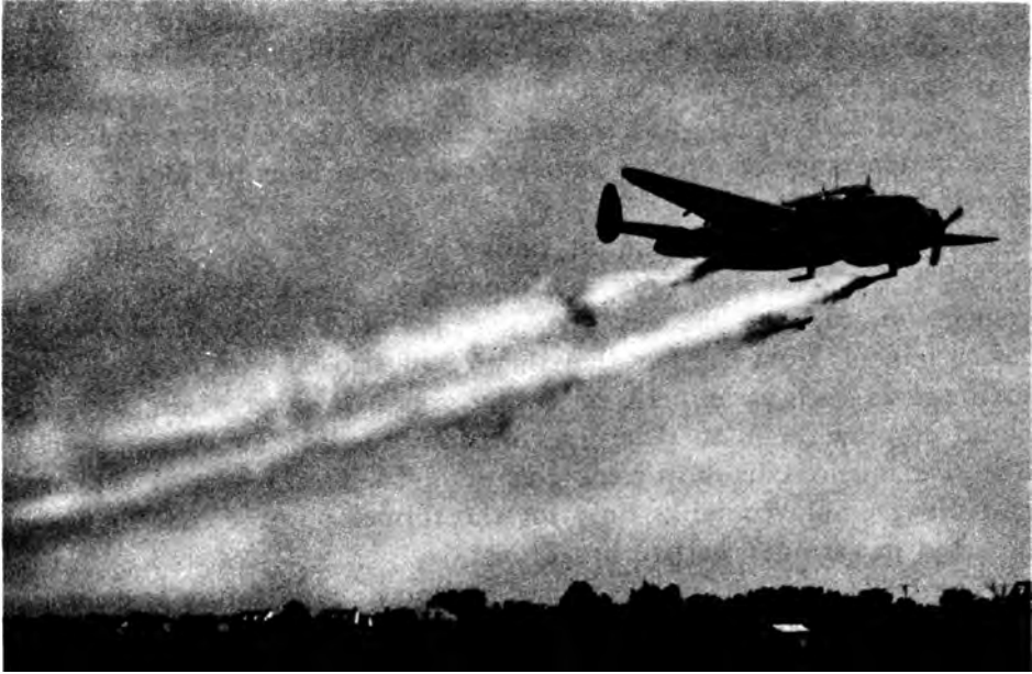
LOCKHEED A-29 SPRAYING SMOKE FROM M33 SMOKE TANKS visible under wings of craft. Smoke tank protruding from bomb bay is the M33 A-1.
