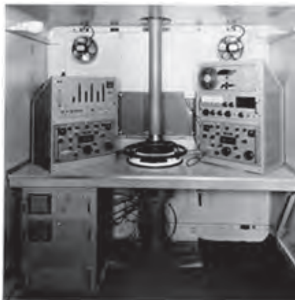
Listening Post. The communications huts associated with the GRAB program amounted to 2,600-pound containers that could be readily transported. Inside was electronic, radio, and recording equipment, as well as an antenna shaft that was rendered steerable with truck steering wheels. (NRL photo Hut_Inside.jpg )
