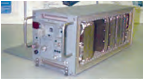
Downsized Tech. By miniaturizing appliance-size Tactical Receive Equipment terminals into the unit shown—the Multi-Mission Advanced Tactical Terminal, or MATT—NRL engineers were able to extend the value of tactical information from satellites and other assets to aircraft. (Source: matt-p1 , Federation of American Scientists )
