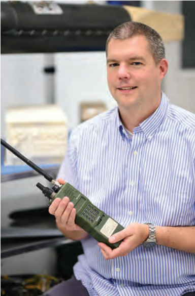
Radio Head. Electronic engineer Chris Huffine shows off hardware from the Software Reprogrammable Payload (SRP) project for which he has led development and testing. SRP relies on software to enable a radio to emulate, and interoperate with, many of the radios in use throughout the military. (NRL photo 140910-N-JF840-003)
