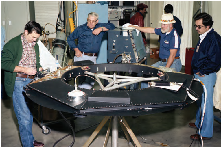
LIPS Service. The first successfully launched satellite in the Living Plume Shield series, LIPS 2, went into space in early 1983. It was developed by modifying a launch vehicle's protective shield that is usually jettisoned in space. The LIPS 2 satellite was used as a demonstration program to prove the capability of the direct downlink of tactical data from a low Earth orbiting spacecraft. The LIPS satellites were designed, built, and tested by the Spacecraft Engineering Department at NRL's Payload Processing Facility. (NRL photo 79878(41).jpg)
