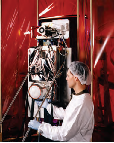
Ion Thrust. NCST engineers prepared this Electric Propulsion Demonstration Module (EPDM) for testing on an NRO technology-testing platform known as Space Technology Experiment (STEx). Referred to as a Hall-effect thruster, it works by ionizing the propellant and then accelerating the ions to create thrust. (NRL photo EPDM.tif)
