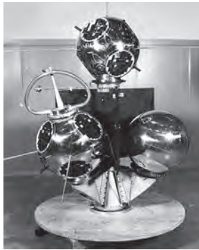
Buckshot. Three portraits, including an artist's rendition and a wooden model, of an ambitious and ill-fated attempt on January 24, 1962, by NRL, along with the Army, Navy, and Air Force, to launch five satellites with a single booster. The cluster was named Composite I, but the nickname Buckshot became its more familiar moniker. (NRL photos 60321.jpg, 60325.jpg, and 60327(2).jpg)
