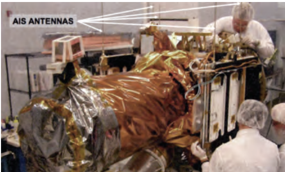
TacSat-2. NCST engineers integrate antennas—including ones that will tap into the maritime system known as AIS, or Automatic Identification System—onto the TacSat-2 spacecraft in preparation for a launch in December 2006.
