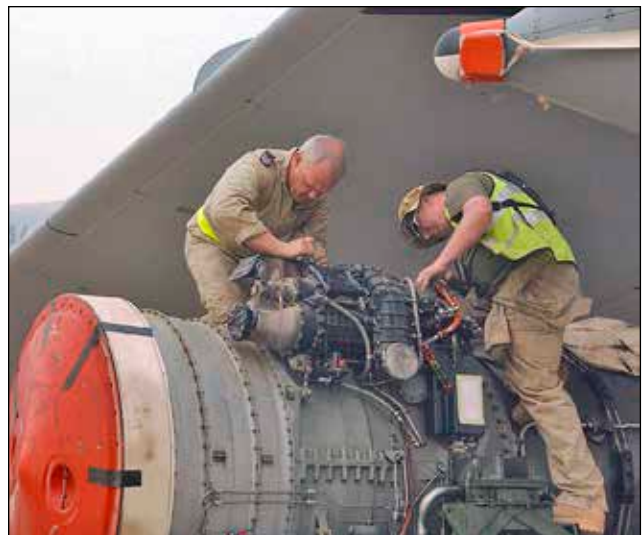
Photo by SSgt Matthew Hannen, USAF. Defense Imagery 030326-F-MY389-002 Sgts David Irland (left) and Gareth Davies, deployed from the Royal Air Force's 101 Squadron, prepare a replacement engine for a Vickers VC-10 C.1K tanker during a fierce sandstorm that began on 25 March.
