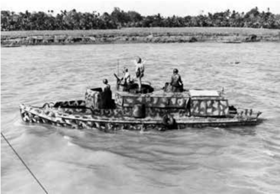
A South Vietnamese STCAN/FOM was a French-designed and -built 36-foot vessel used by the Vietnam Navy for river patrol, fire support, and minesweeping.
