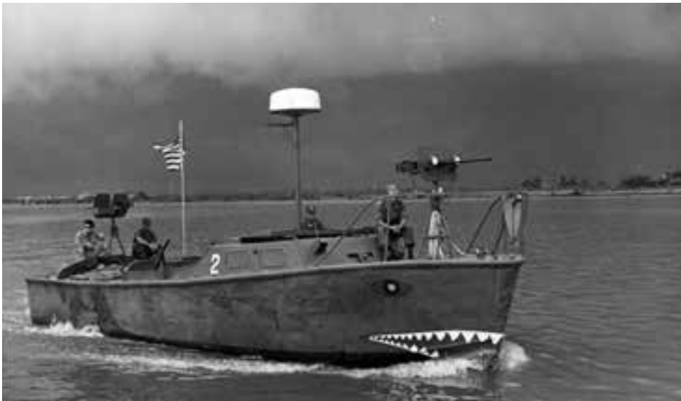
LCPL on the Saigon River, October 1965. These 36-foot-long patrol boats provided security for the Saigon shipping channel prior to the arrival of the PBRs.
