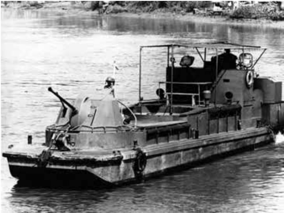
A Vietnamese Navy LCM monitor conversion armed with a .50-caliber machine gun, 20mm and 40mm cannons, and an 81mm mortar, 31 August 1964.
